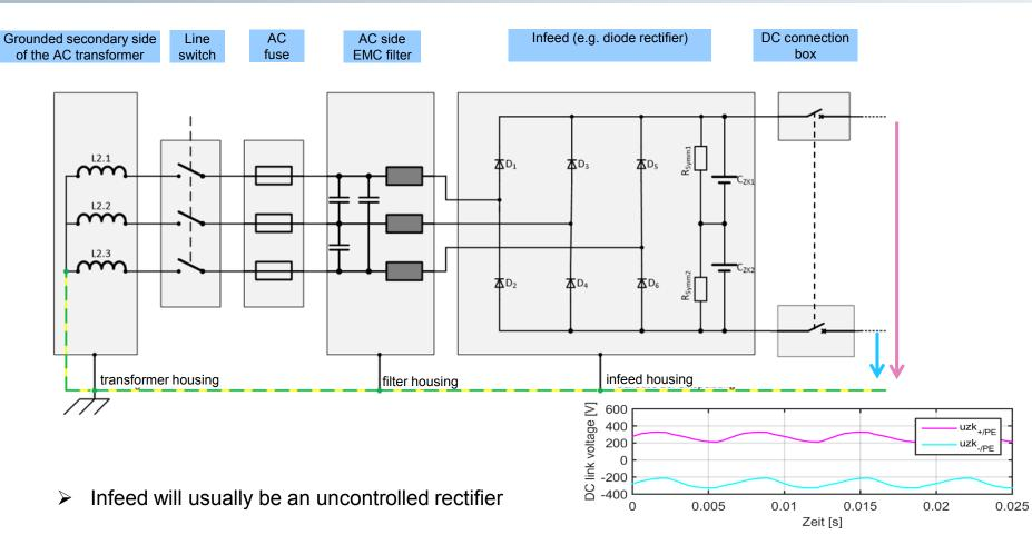
> DC voltage to ground is impressed, both DC lines require a protective device.
