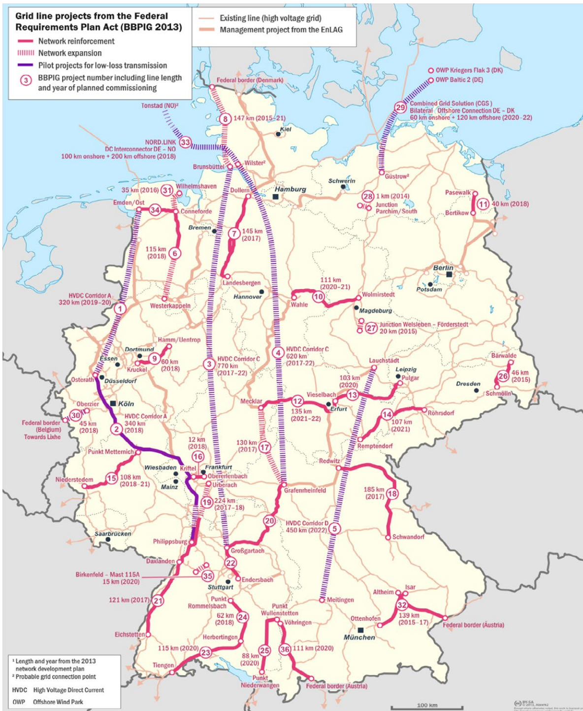
Figure 6 The planned expansions and reinforcements of the German high voltage power grid (200 kV+) (Alexrk2, 2013) (translated)
