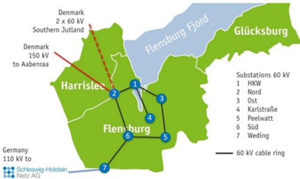
Figure 14 The supply area of Stadtwerke Flensburg, the 60 kV cable ring system and the connections to the German and Danish high voltage grid (Stadtwerke Flensburg, 2020a) (translated)
