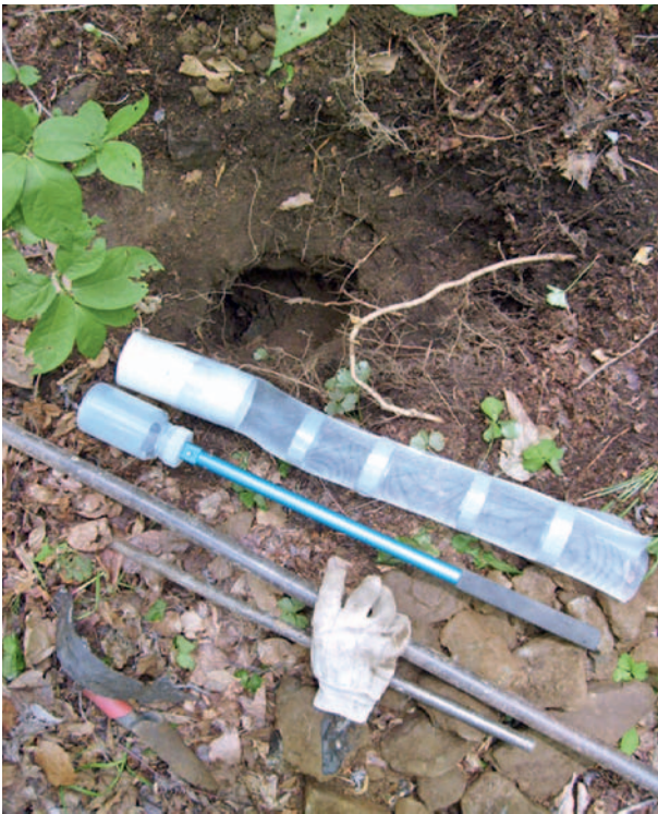
Fig. 3. Deep soil trap inspired by THOMPSON (1995) and used in the Russian Far East for the endogean fauna. Both Fusi and Sciaphyes were collected with this type of trap. This trap, once set up, might be serviced as often as desired by means of retreating the deeply sunk collecting jar with the aid of a screw lid firmly attached to the extended handle. The mesh allowed the beetles to crawl through and fall into the jar filled with glycerol (ethylen glycol or a saturated water solution of table salt are suitable alternatives). It was found that the mesh sleeve is too weak to keep its shape for more than a year and, therefore, a solid plastic sewage pipe some 30–40 cm long with numerous drilled holes should be preferably used. For an alternative strategy of deep soil trapping see GIACHINO & VAI-LATI (2010).
