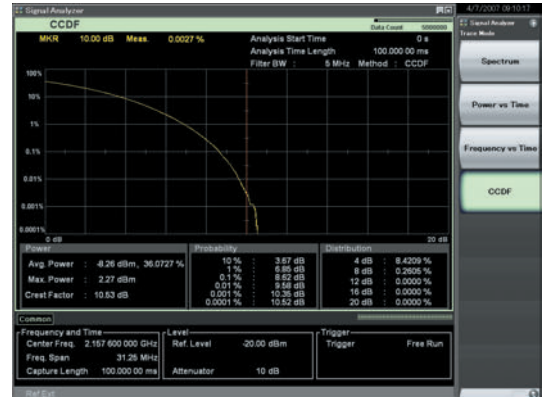
CCDF (Test Model 1, 64 DPCH, 1 Carrier) Waveform Pattern [Test_Model_1_64DPCH]
