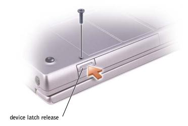
**6** Pull the device out of the module bay.
