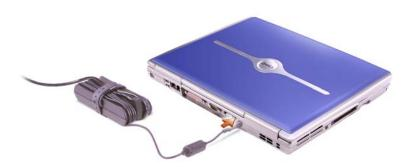
The AC adapter converts AC power to the DC power required by the computer. You can connect the AC adapter with your computer turned either on or off.
