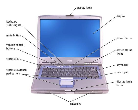
**DISPLAY LATCH** — Keeps the display closed.
