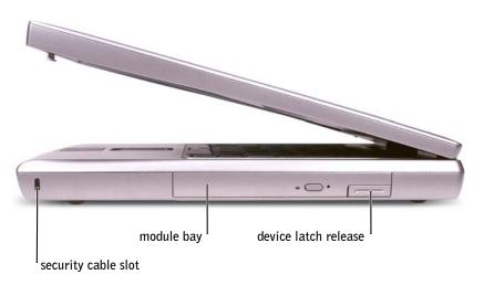
SECURITY CABLE SLOT — Lets you attach a commercially available antitheft device to the computer. For more information, see the instructions included with the device.
