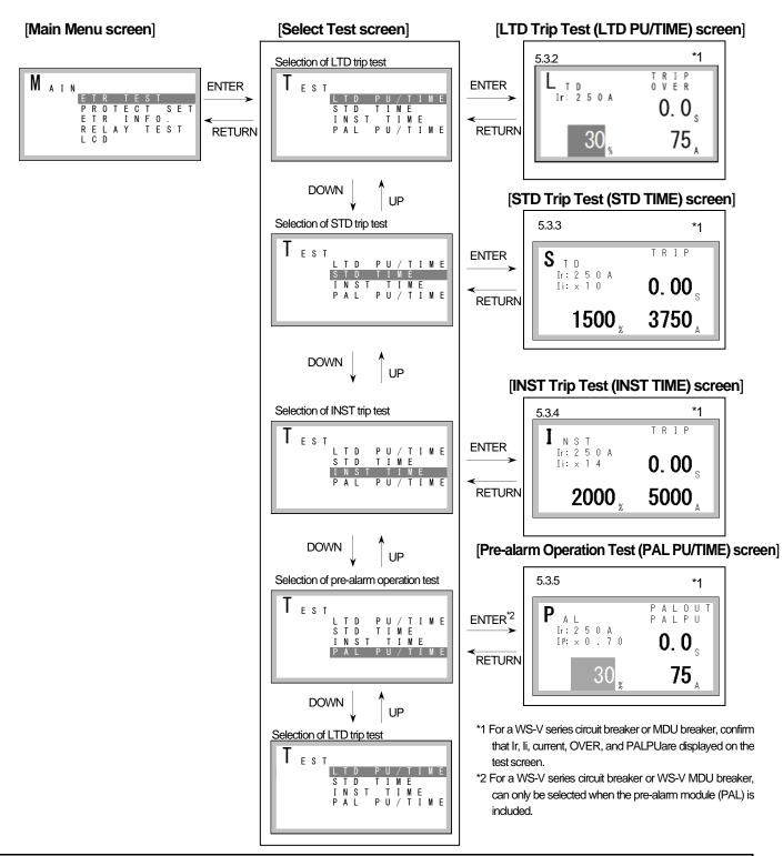
Do not trip test the main circuit of a circuit breaker with voltage applied. This leads to the dangerous state where the circuit breaker trips or an arc is generated.
