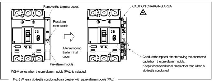
$r_{1}$ ,  $\sigma$  which a trip test is conducted on a breaker with a pre-alain module (r AL)
