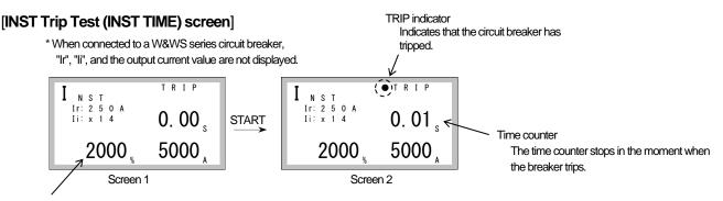
Current signal level Fixed to 2000% of the rated current, and cannot be changed.
