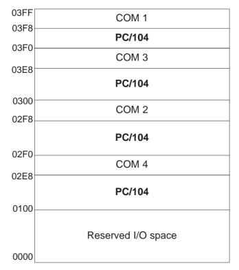
The PC104 bus is accessed via I/O reads from and writes to PC/104 addresses shown in the table on page 10.
