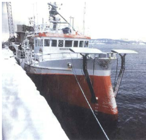
Figure I.2.1-5 Norwegian ship achieves fuel savings 15-20% by wave-energy extraction, Jakobsen (1983)
