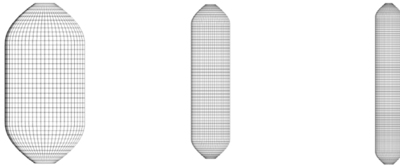
Figure III.1.1-7 Wing outline for s/c = 2, 4, 6 respectively.
