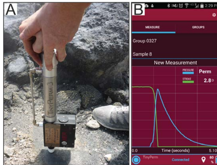
Figure 3.6: (A) Portable permeameter TinyPerm III during field measurement and (B) TinyPerm app on an Android device permitting wireless data collection.
