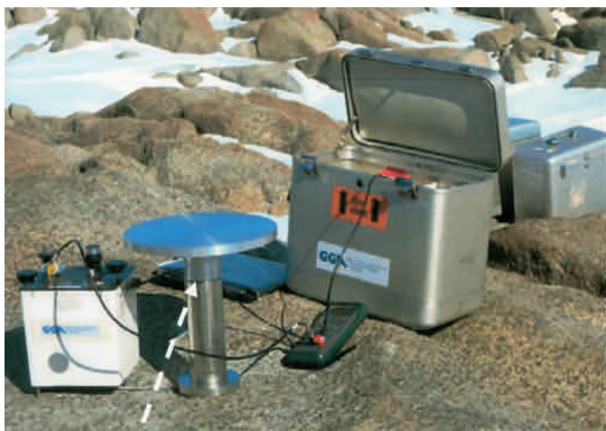
Fig. 2: Measurements at point VL15, Inexpressible Island. The table proved to be not usable due to unexpected vibrations. Here, G-662 is seen, the other two gravity meters are in the boxes behind. The arrow points to the top of the benchmark as the reference, (Photo: author).
