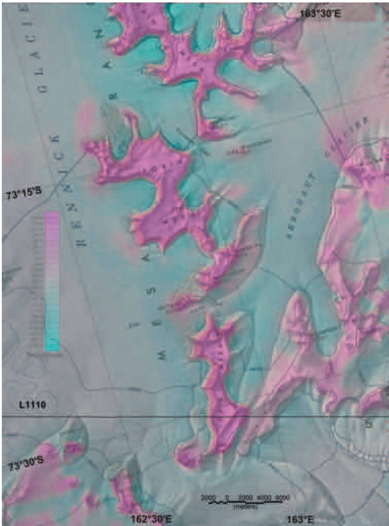
Fig. 10: The anomalies of the total magnetic field superimposed on the topographic map (section of the USGS Topographic Reconnaissance Map (250K) Mount Murchison). Colour scale is equal-area. The flight path for line L1110 is marked.
