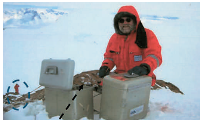
Fig. 4: Measurements with G-858 at Mt. Jiracek (VL08). The boxes of the other gravimeters are used as windshields, the arrow points to the top of the benchmark. Circled below left is the helicopter pilot worrying for a developing whiteout, which appeared only some minutes later and forced us to abandon the measurement. The position of the pilot reveals that the climb up-hill was not that easy, (Photo: private).
