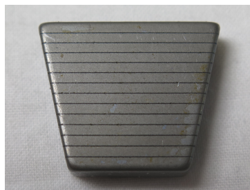
Figure 5.5: Segmented magnet used in the prototype motor
