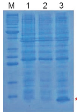
Fig. 2 Overexpression of a heterologous protein (ubiquitin) using the SPP system, confirmed by SDS-PAGE. The gel was stained with Coomassie Brilliant Blue. The red asterisk indicates the position of ubiquitin band. M, molecular weight markers. Lane 1 , before the induction of MazF and ubiquitin expressions; Lane 2 , after the induction of MazF expression without ubiquitin; Lane 3 , after the induction of ubiquitin expression
