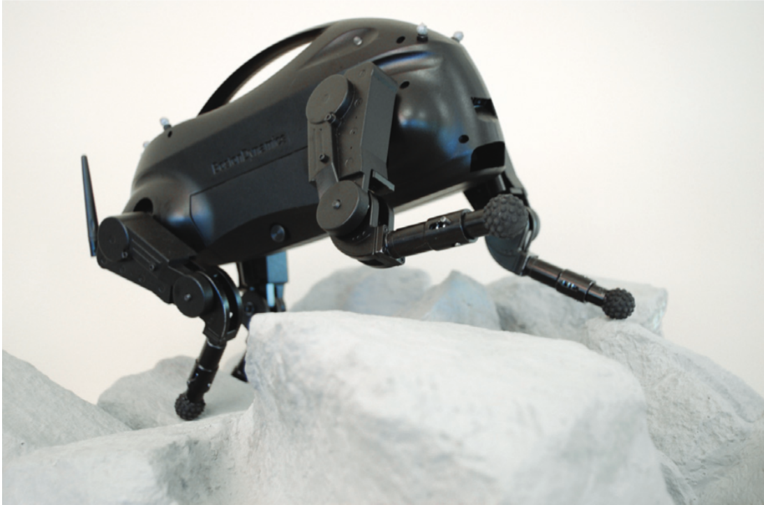
Figure 1.1: Little-Dog, a quadruped bio-inspired robot produced by Boston Dynamics Incorporated. [4]
