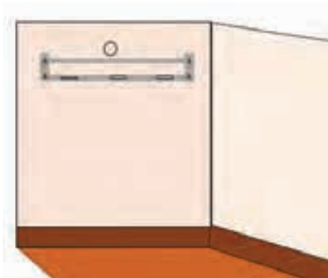
Fig. 4.4.3.4t: Drill a hole for piping
