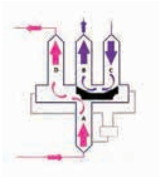
Fig. 2.3.4.1: A four way valve in cooling mode
