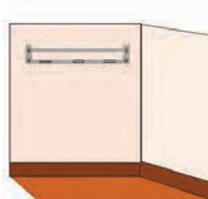
Fig. 4.4.3.3: Secure the mounting plate
