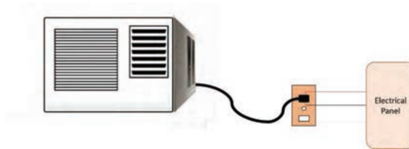
Fig. 4.3.1.1: Wiring diagram of a window AC
