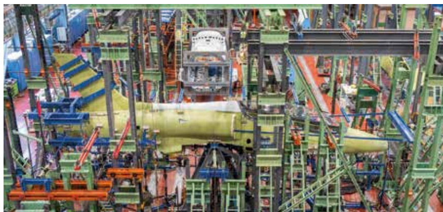
An AERO L-39NG undergoing a stress test
