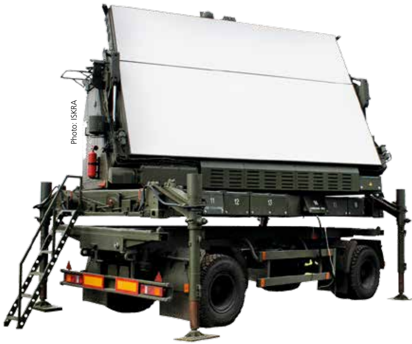
The mobile 90K6E 3-D air surveillance radar with transistorised transmitter for low, medium and high flying target detection
