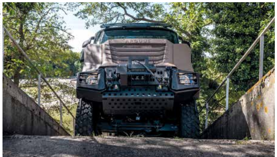
The Arquus ARMIS 6x6 climbs a 50% slope at the Satory test track in September during a demonstration. The ARMIS family has three variants: 4x4, 6x6 and 8x8. Arquus believes that the ARMIS family is the ideal choice for the future French Army truck requirement.
