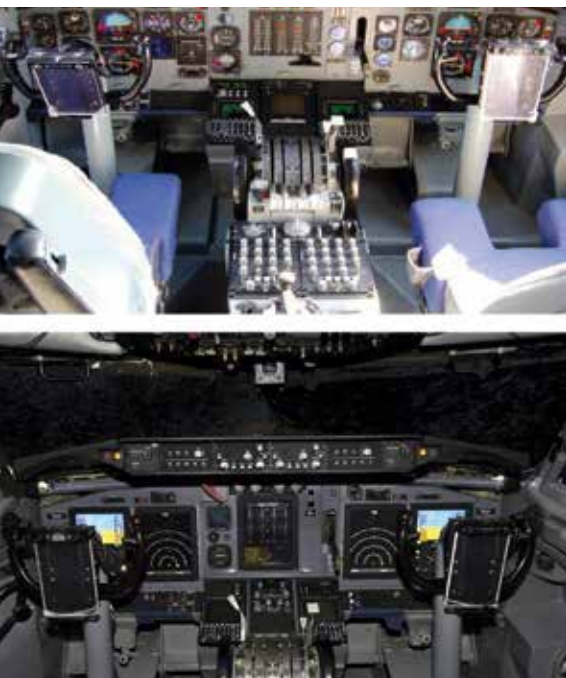
In 2015, NATO's E-3A (NE-3A) aircraft were upgraded with glass cockpits and other advanced avionics to meet current and future Communication, Navigation, Surveillance / Air Traffic Management (CNS/ATM) airspace requirements.
