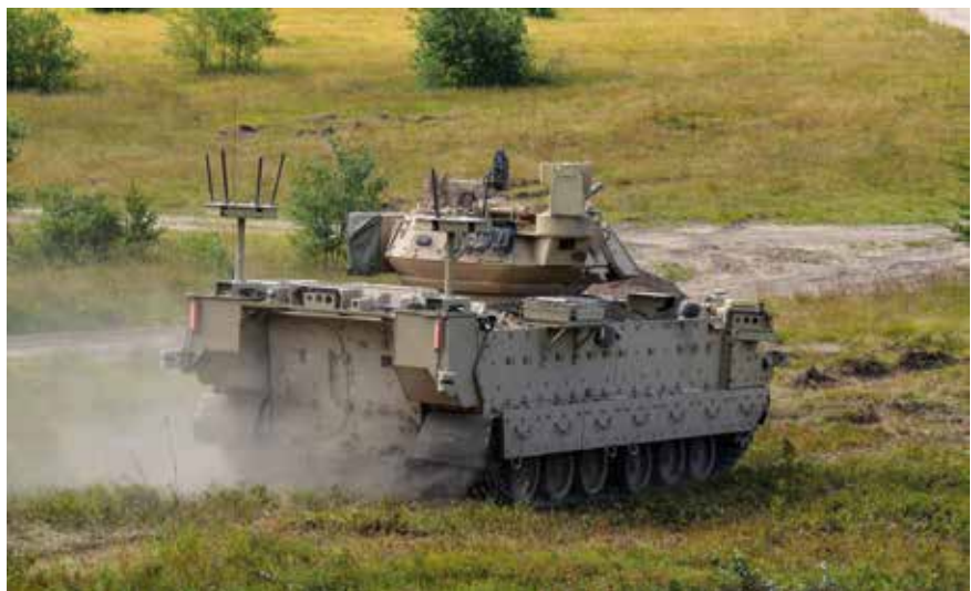
The MET-D based on a modified M2 BRADLEY at robotic vehicles tests at Ft. Carson
