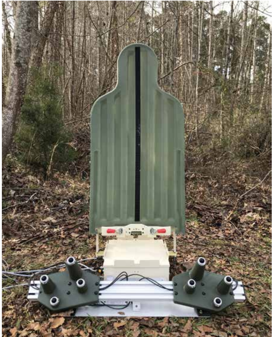
A LOMAH device fitted to a pop-up target
