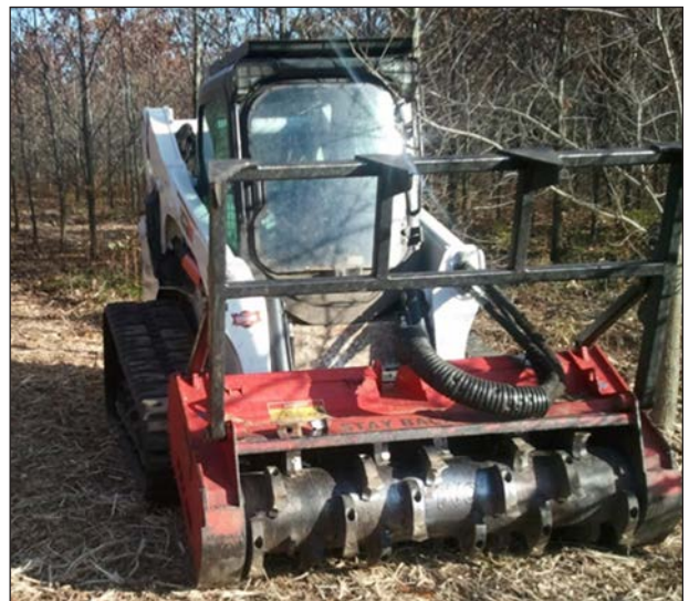
Figure 23. Rotary grinders and other clearing equipment may be used to start control of dense tree-of-heaven patches, but follow-up herbicide applications will be needed to control the root and stump sprouts resulting from this treatment. Photo by Lenny Farlee
