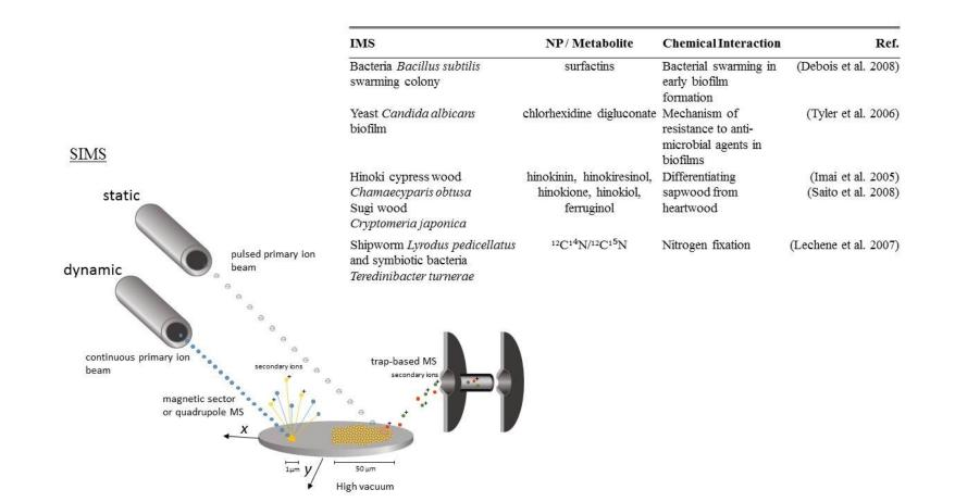
Figure 1.7 Secondary mass spectrometry (SIMS) imaging methods with examples of natural product and chemo-ecological studies (adapted from (Bouslimani et al., 2014, Bergman et al., 2014, Watrous and Dorrestein, 2011, Esquenazi et al., 2009, Saito et al., 2008).
