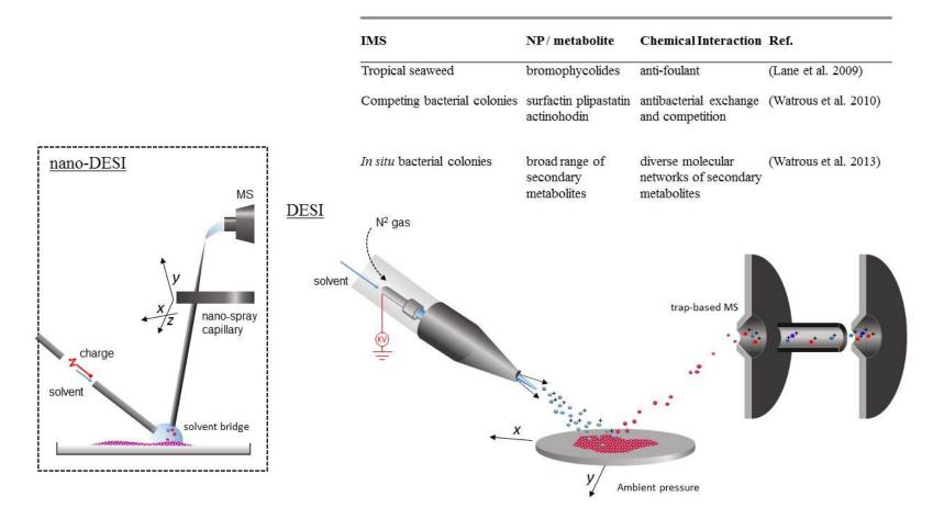
Figure 1.6 Ambient desorption electrospray ionisation (DESI) and nanoDESI mass spectrometry imaging methods with example natural product and chemo-ecological studies (adapted from (Bouslimani et al., 2014, Bergman et al., 2014, Watrous and Dorrestein, 2011, Esquenazi et al., 2009).
