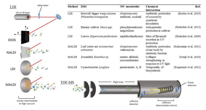
**Figure 1.5** Laser desorption ionisation (LDI) and matrix assisted-LDI (MALDI) mass spectrometry (MS) imaging methods and schematic of time of flight (TOF) analysis with example natural product and chemo-ecological studies (adapted from (Bergman et al., 2014, Watrous and Dorrestein, 2011, Esquenazi et al., 2009, Bouslimani et al., 2014)
