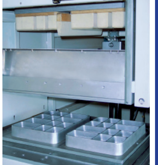
thermoforming of parts with pre-stretcher
