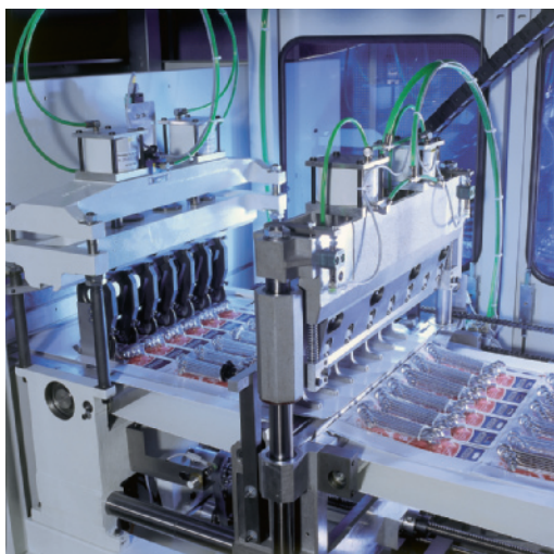
SB 74e-3 and SB 74e-4 longitudinal and cross cutter with quick-change technology of longitudinal knives
