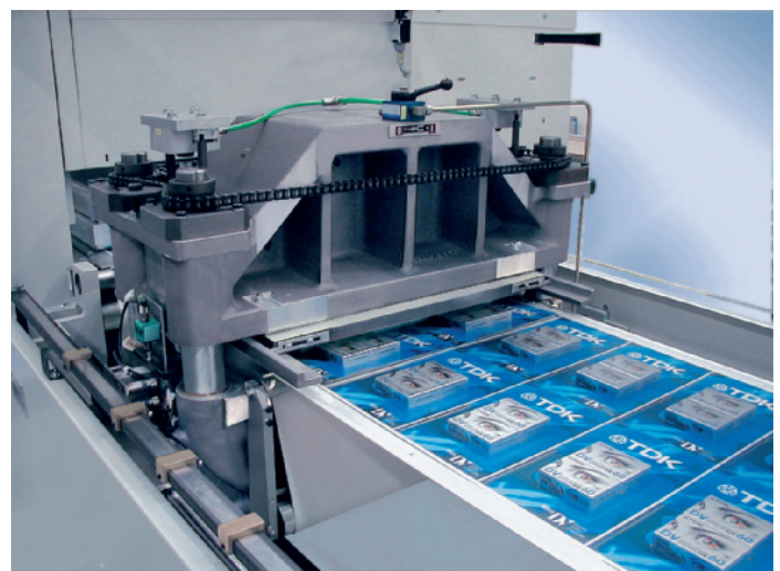
enhanced packs SB 74e-9 and SB 74e-10 contour cuts with steel rule punch press
