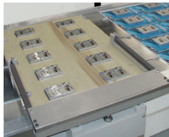
positioning of goods by means of loading template
