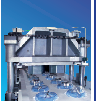
steel rule punch press of contour cuts
