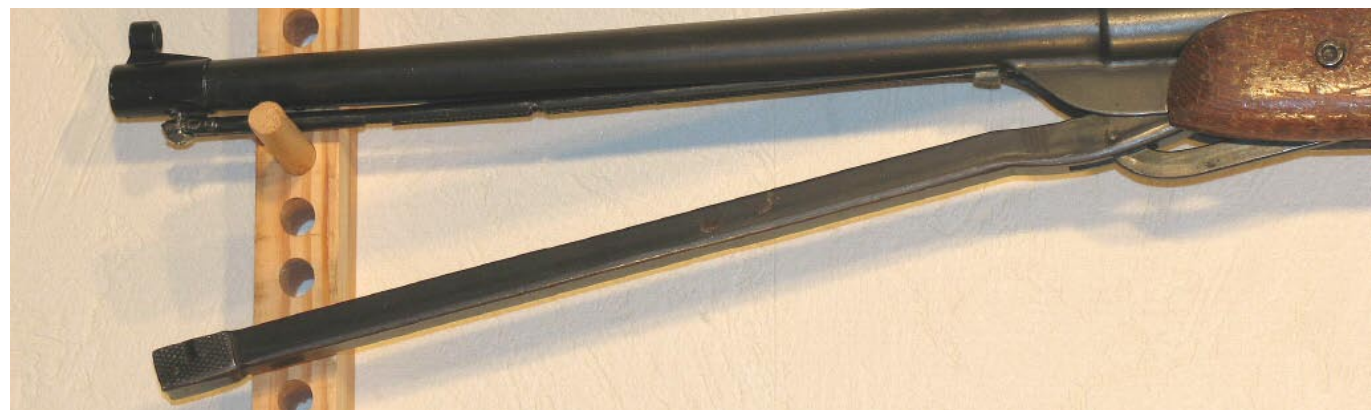
CondoRifle: underlever cocking with magazine hidden under barrel
