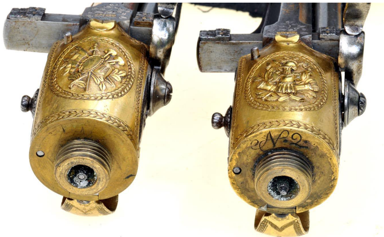
Figure 7: With the grip reservoirs removed, the pistol markings on the number 2 specimen can be seen. Also visible is the firing pin positioned within the centre of the air passage cavity in the receiver. A close inspection at the 9 o'clock locations on the receiver faces will reveal the locking pin for the reservoir.
