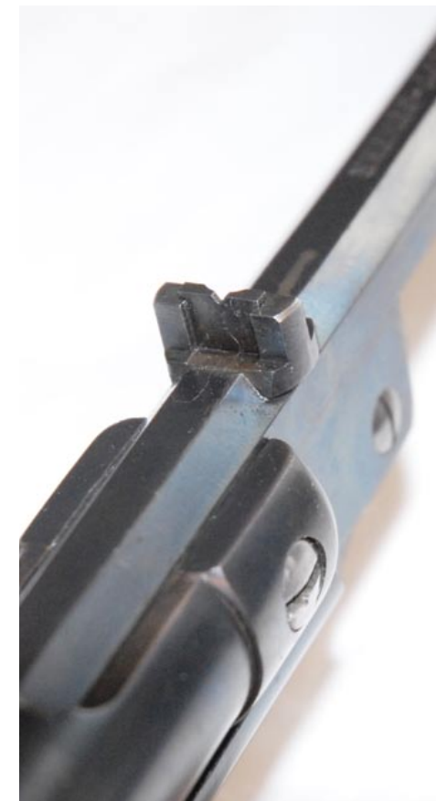
The adjustable gate rear sight may have been installed as an upgrade
