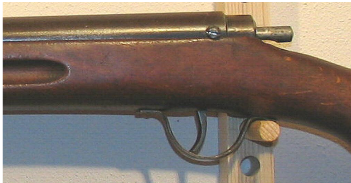
The Hubertus has a protruding piston rod when cocked – a nice detail.
