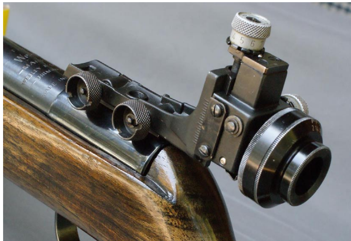
Anschutz 6706 rear diopter sight with contemporary Anschutz-made iris
