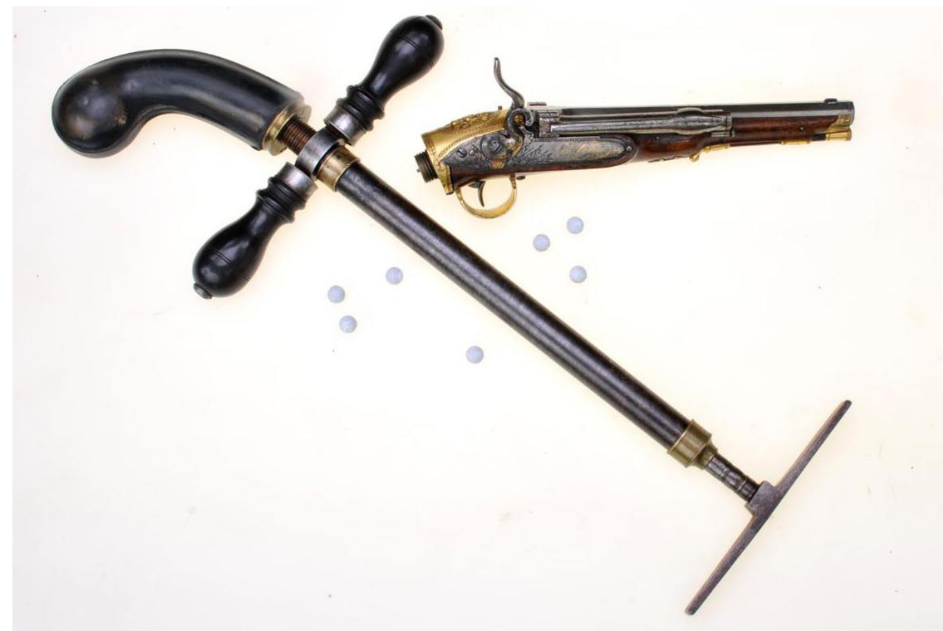
Figure 9: Once the grip reservoir is removed from the pistol, it is threaded onto the top of the pump above the ebony handles. The small steel plate is placed beneath the shooter's feet to secure the pump during the air charging procedure.
