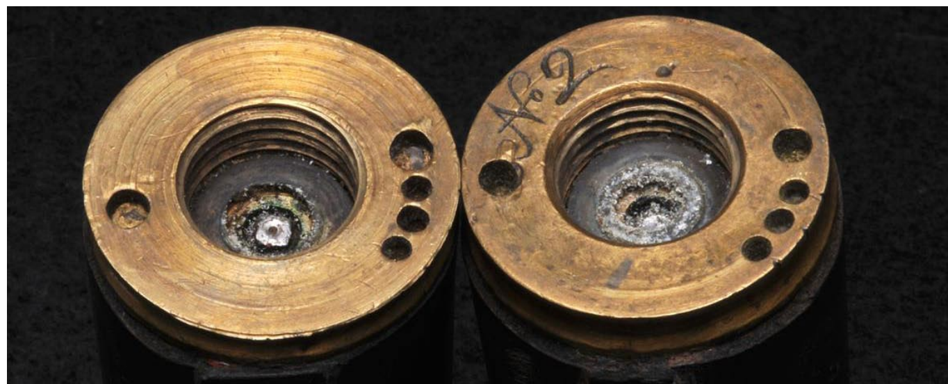
Figure 8: The front faces of the grip reservoirs are each drilled with three holes to allow the indexing and anchoring of the grips to the receivers.
