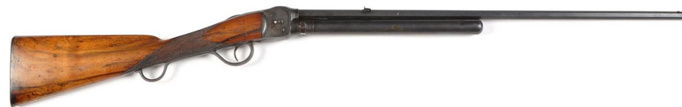
Giffard set up in London and produced this CO2 rifle. An under lever opened the breech loading port
