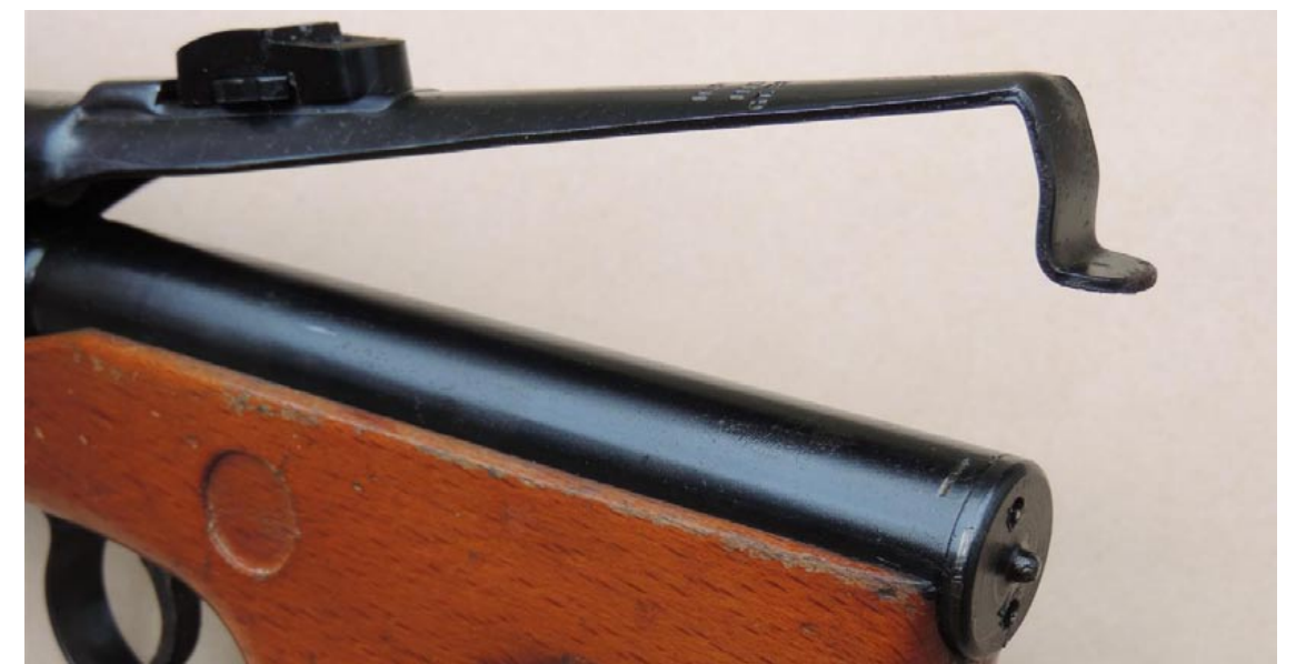
The screw in end cap can be seen on this mid 1970s G4
