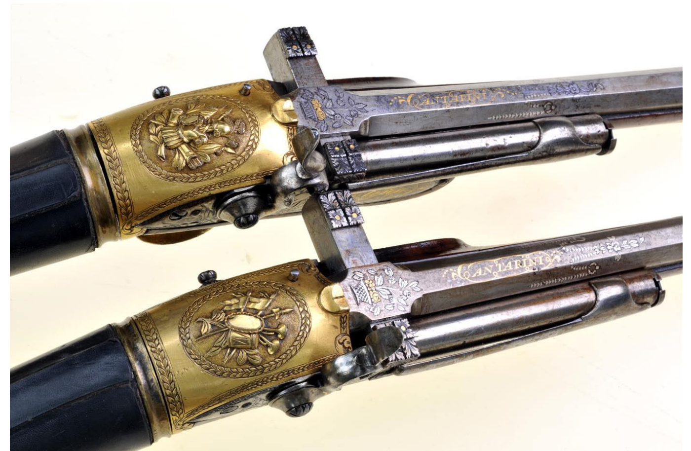
Figure 4: Both air pistols are essentially identical in appearance, with only a few small detail differences seen in the decorations. The coats of arms seen at the top of each receiver are slightly different in theme. Please note the 10-shot magazine affixed to the right side of each pistol.
