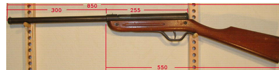
CUNOX sliding breech underlever rifle
