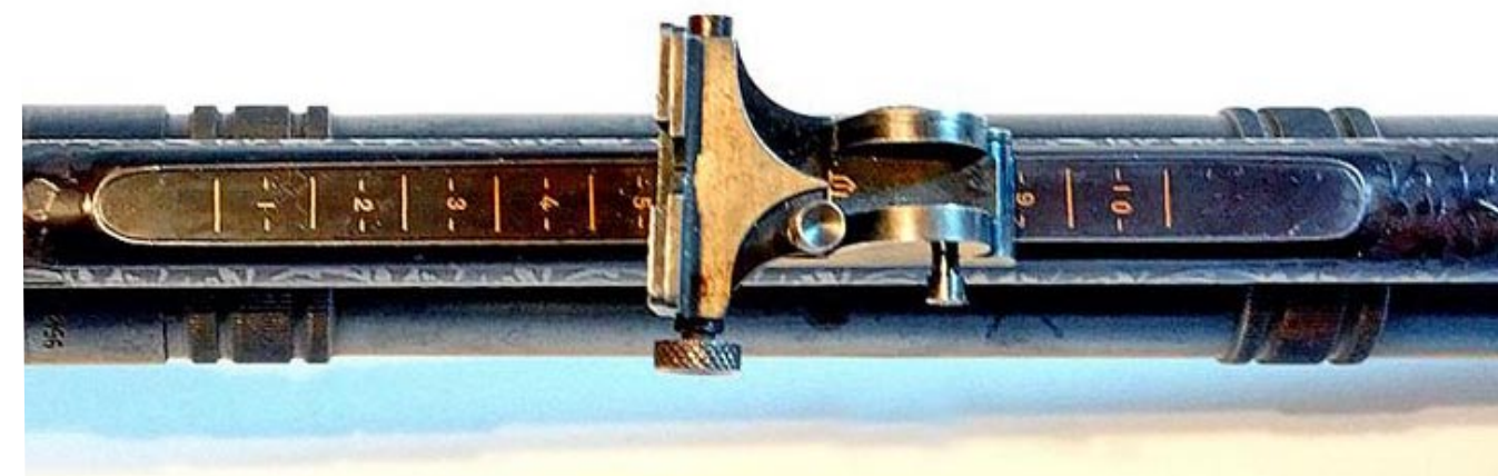
The 'match' Giffard rear sight could be moved along a rail to adjust eye relief (photo courtesy of B McKenzie)
