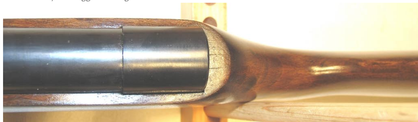
Breda Arill square triggerhousing with beech stock and no medallion in the stock (cylinder end cap detail)
