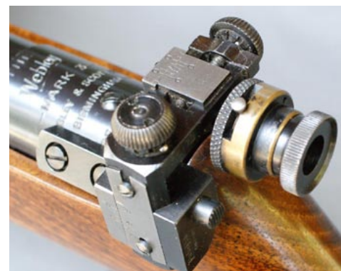
The PH 'Iris' infinitely-variable eyepiece
