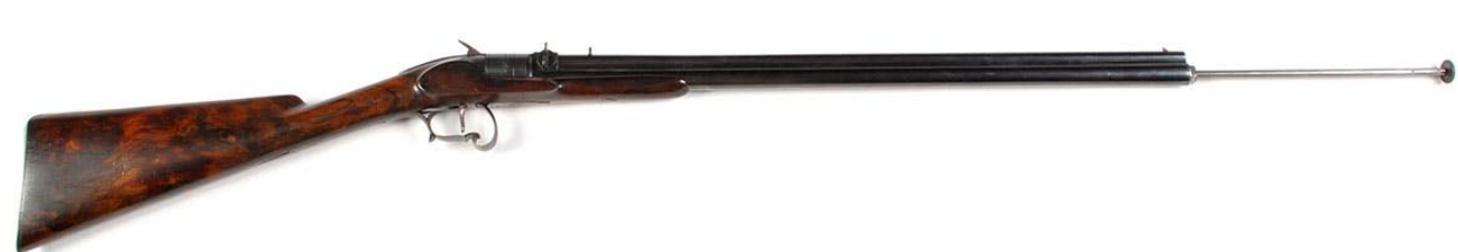
Giffard in-line pump pneumatic rifle
