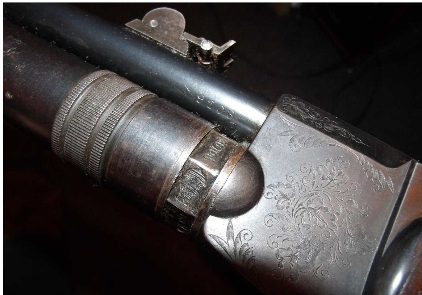
Cartouches were often damaged due to tightening with the wrong spanners
