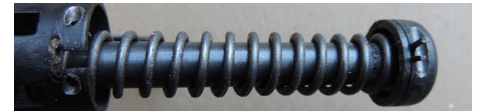
There is significant mainspring preload on the Mark IV
