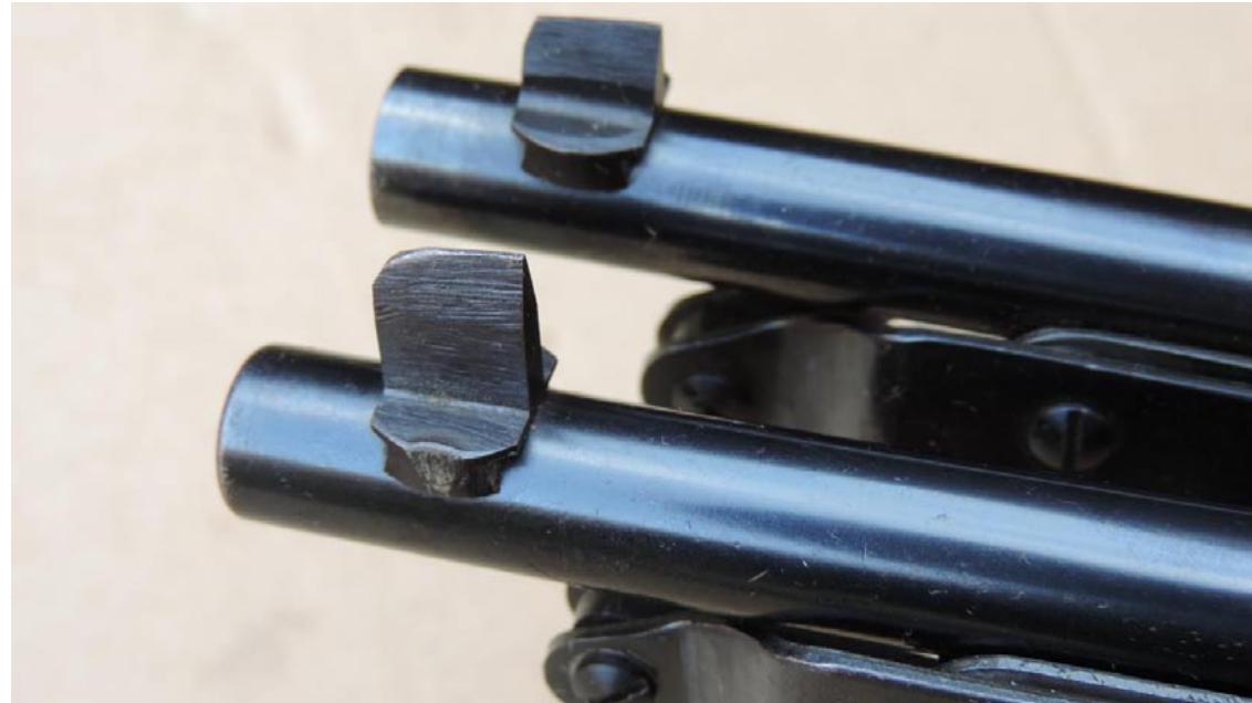
Early (top) and late knife profile foresights. The late sight is scarce
