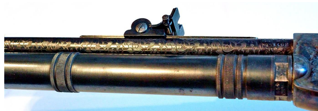
Giffard CO2 rifles had a precision adjustable rear sight, shotguns had a simple blade (photo courtesy of B McKenzie)
