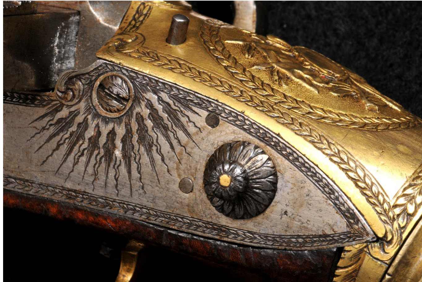
Figure 10: The small engraved button near the back of the sideplate is used to anchor and index the grip to the shooter's preferred angle. The bypass button (rod) can be plainly seen protruding from the top of the receiver.
