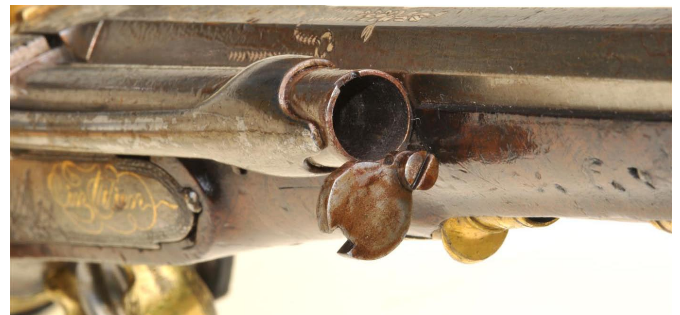
Figure 11: The pivoting door at the front of the magazine tube is swung open to allow the loading of ten .40 caliber lead balls. The small (and fragile) spring retainer holding the cap in position is missing from both specimens.
