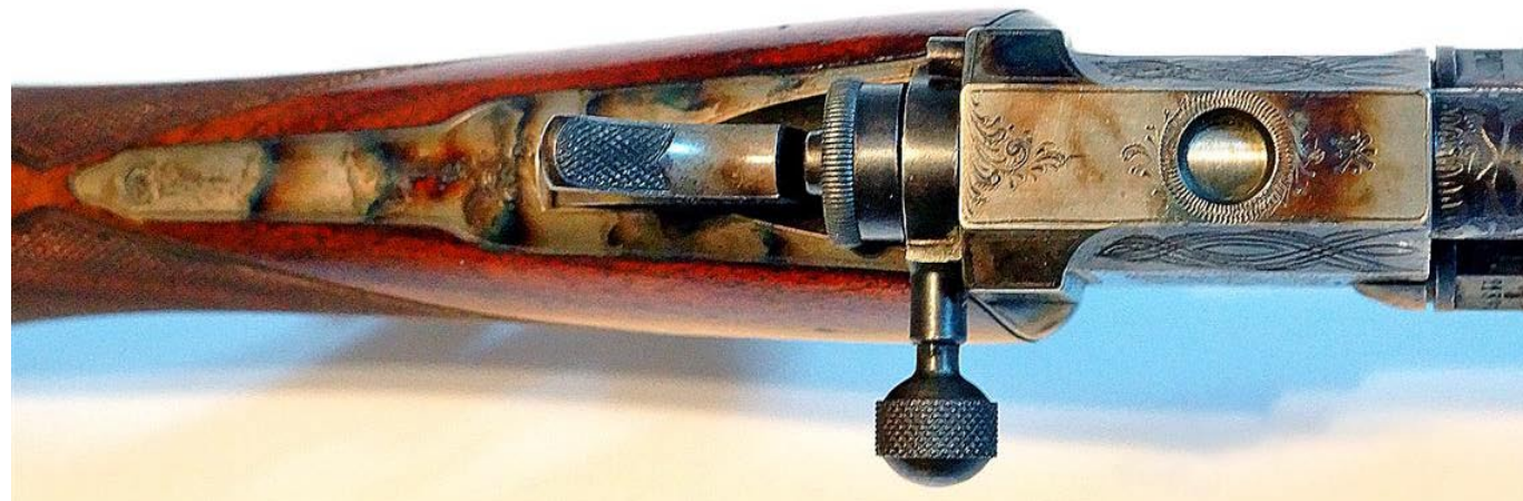
The most common CO2 Giffards used a bolt breech loading system (photo courtesy of B McKenzie)
