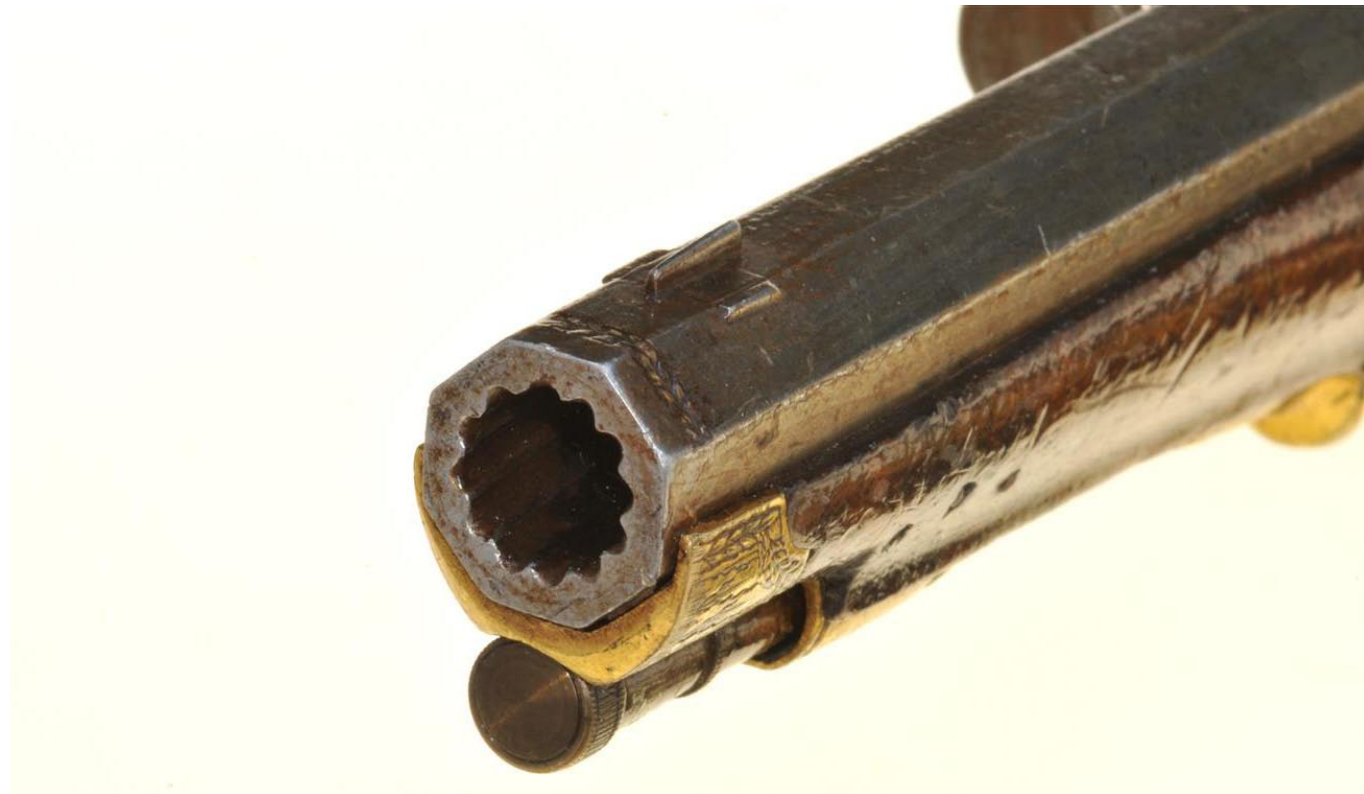
Figure 12: The muzzle of the Austrian repeating air pistol reveals a very impressive set of deep rifling within the .40 caliber bore.
