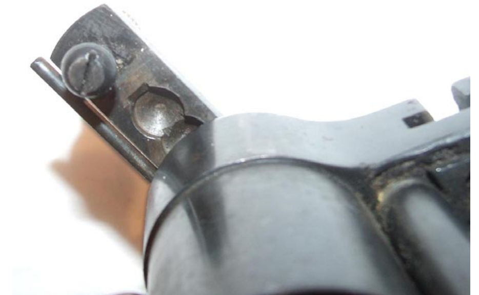
Breech cover open (air transfer depressions visible)
