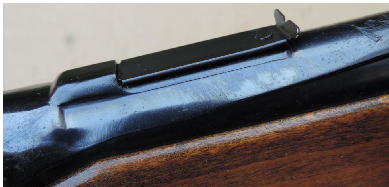
A non-adjustable rear sight from a 1964 dated Mark IV
