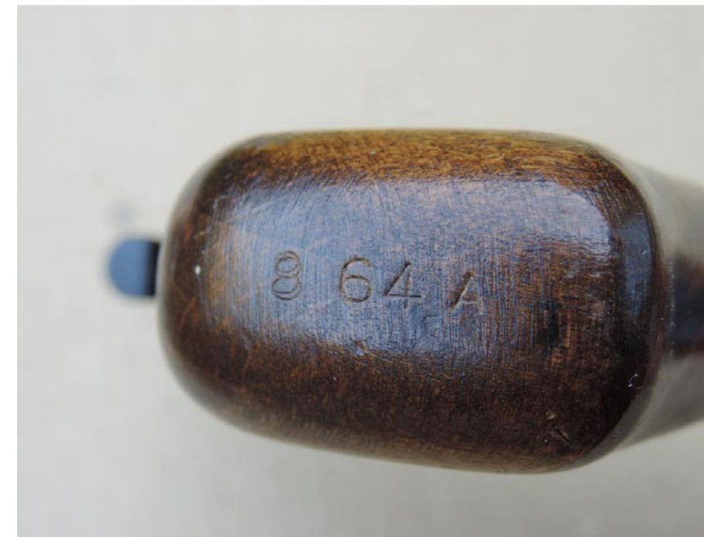
Date codes were stamped on the base of the grip until the 1970s
