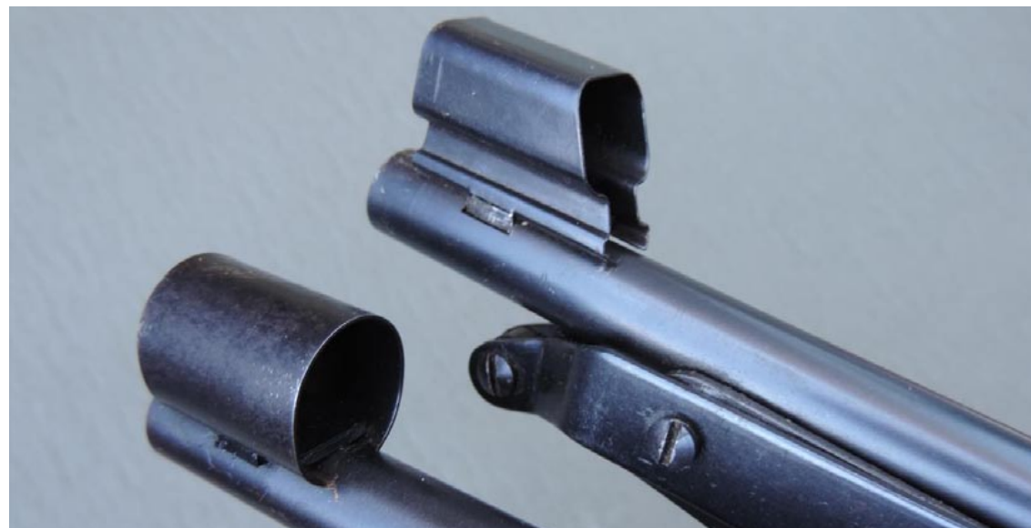
The early pillar foresight (top) had a more angular hood than the later variant
