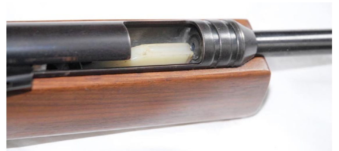
Anschutz LG220 breech with pop-up pellet 'bridge'
