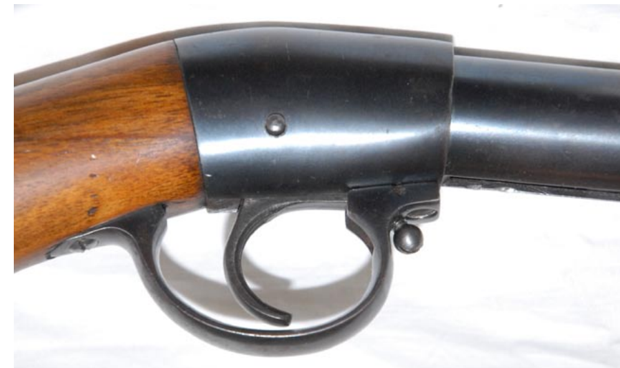
The trigger block and guard show no sign of manufacturing economies
