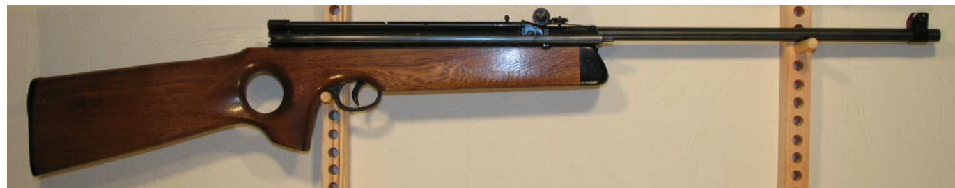
Mahely, made by Industria Argentina. A rare combination of features: thumbhole stock, sidelever cocking, tubular magazine, and swing-out loading gate.
