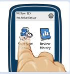
Touch **Start New Sensor**. Hold Reader within 1.5 inches (4 cm) of Sensor to scan it.
