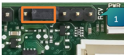
Figure 3 Config pin header (> K39xx) -> Pin 5+6
