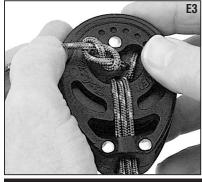
E3 Tie a loose figure eight knot. Move knot so it is tight against block. Leave at least 25mm (1") of line beyond knot. Repeat for other line end. Trim excess line.
