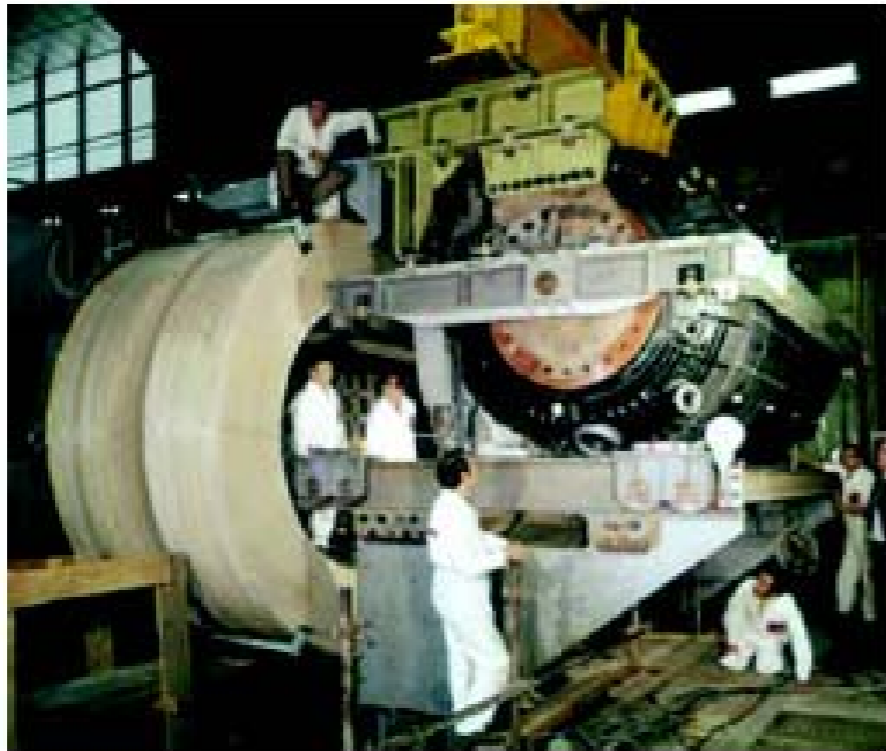
Fig. 1: The Gargamelle heavy-liquid bubble chamber, installed into the magnet coils, at CERN in 1970.
