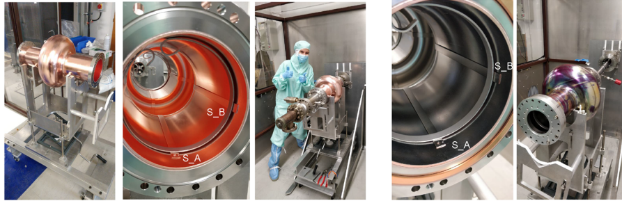
Figure 4.15. First Nb thin-film-coated 802 MHz cavity at CERN. The three leftmost figures show the copper cavity before coating including the clean-room assembly. The two rightmost figures show the cavity after the Nb coating [243].
