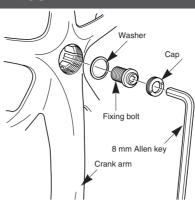
The crank arm can be removed simply by turning the fixing bolt counterclockwise.
