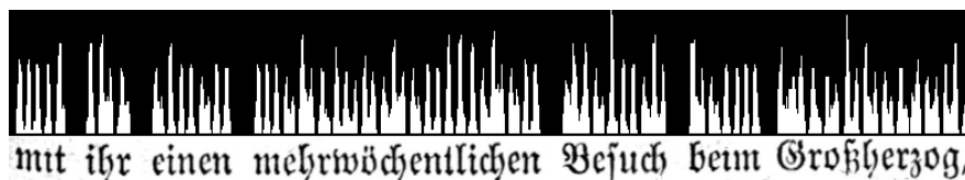
Fig. 10: Original text line and its vertical projection profile.
