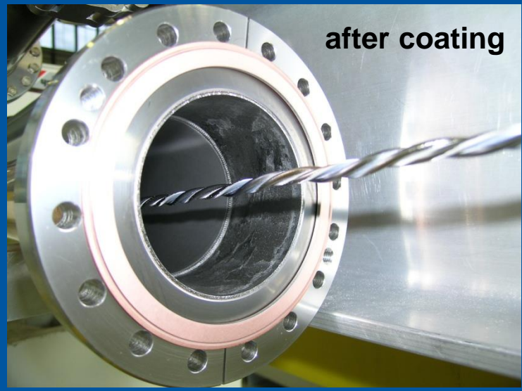
Cross section of the LHC warm dipole vacuum chamber
