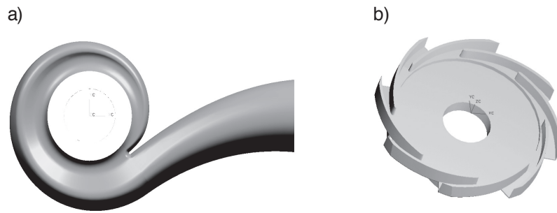
Figure 1.5: Common stationary collector geometries in centrifugal pumps
