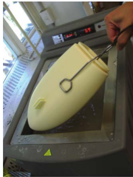
(b) Dissolving support material in alkaline bath (the main body of UC-Ika 1)
