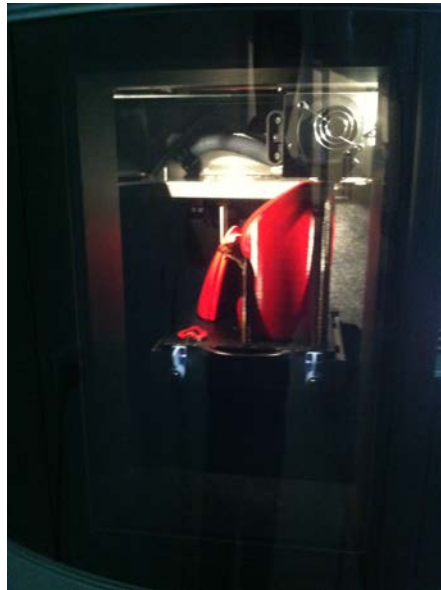
(a) The main body of UC-Ika 2 in 3D printing machine
