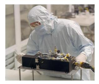
ALICE is imaging spectrograph in the  $\lambda\lambda70-205$  nm,  $\Delta\lambda$  0.8 -1.2 nm. The slit, 5.5° long, with a width of 0.05° - 0.10°. Alice employs an off-axis telescope feeding a 0.15-m normal incidence Rowland circle spectro-graph with a concave holographic reflection grating. MCP detector utilizes solar-blind opaque photo-cathodes (KBr and CsI).
