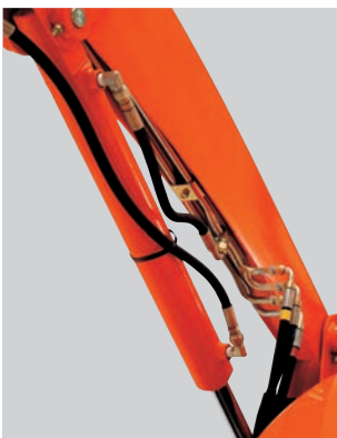
Protected Cylinder Tubes
