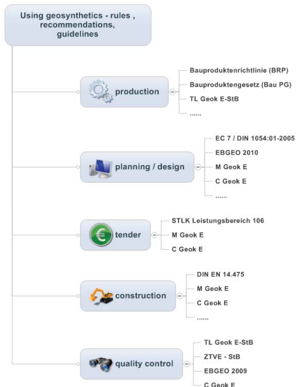
Fig. 13 From production to quality control with geosynthetics
