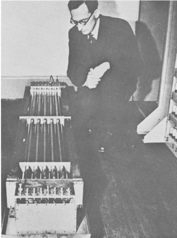
Fig. 3 Wilkes and his mercury delay line memory.
