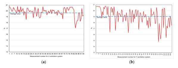
**Figure 12.** Changes in concentrations of oxygen in the goaf air—the U-type (**a**) and the Y-type ventilation system (**b**).
