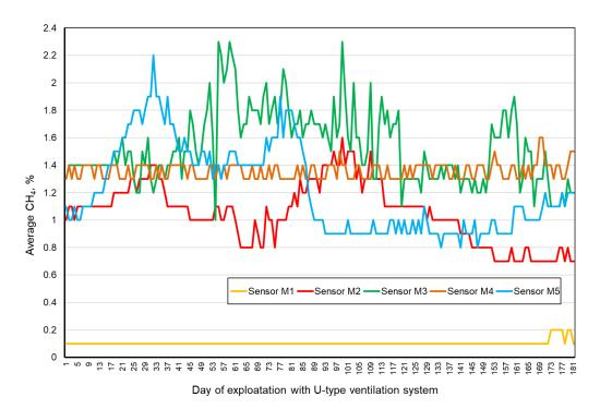
Figure 7. Registered concertation of methane for the U-type ventilation.
