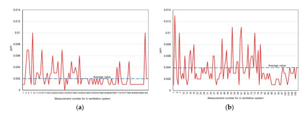
**Figure 17.** Changes in concentrations of acetylene in the goaf air—the U-type (**a**) and the Y-type ventilation system (**b**).
