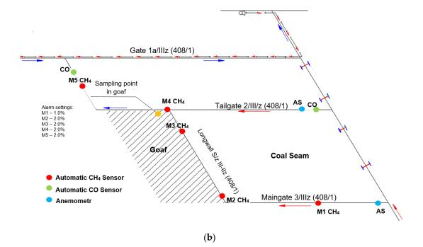
Figure 6. Diagrams of the tested longwall for the U-type (a) and Y-type (b) ventilation systems.
