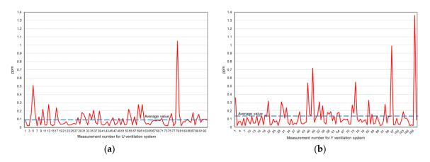
**Figure 19.** Changes in concentrations of propane in the goaf air—the U-type (**a**) and the Y-type ventilation system (**b**).
