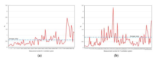
**Figure 14.** Changes in concentrations of carbon dioxide in the goaf air—the U-type (**a**) and the Y-type ventilation system (**b**).
