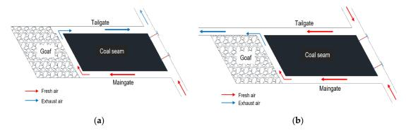
**Figure 1.** Diagram of the U-type ventilation system (**a**) and the Y-type system with routine ventilation of tailgate (**b**).
