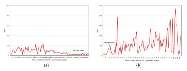
**Figure 13.** Changes in concentrations of carbon monoxide in the goaf air—the U-type (**a**) and the Y-type ventilation system (**b**).
