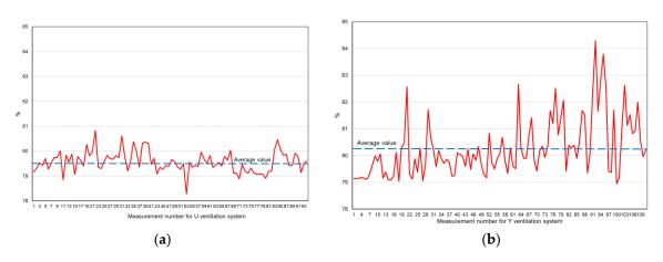
**Figure 20.** Changes in concentrations of nitrogen in the goaf air—the U-type (**a**) and the Y-type ventilation system (**b**).
