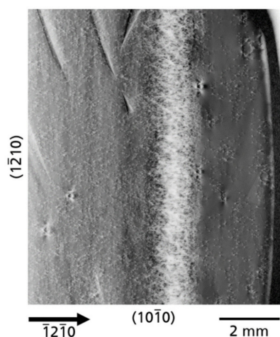
Figure 10. XRT image using \bar{1}2\bar{1}0 reflection with a wall of a dense dislocation network observed in crystal A. The Borrmann effect is nearly extinct for this highly defective region.
