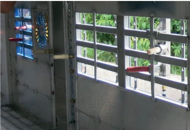
Fig. 7: Metal nipple device covered in plastic
