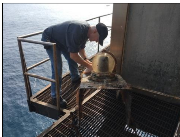
Richard Neal examines the fouling on SharkCam after removal in January 2017. Image credit: David Wood
