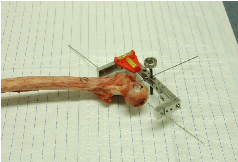
Fig. 4-4. Defining the first reference plane. The femur lies on its three natural landmarks (lesser trochanter and condyles). The tool is attached to it and the second axis leveled. A third reference point is marked out on the femoral neck.
