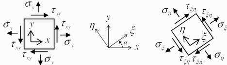
$$\underline{T}_{xy} = \begin{bmatrix} \sigma_n & \tau_{xy} \\ \tau_{xy} & \sigma_y \end{bmatrix} \quad \underline{T}_{\xi\eta} = \begin{bmatrix} \sigma_\xi & \tau_{\xi\eta} \\ \tau_{\xi\eta} & \sigma_\eta \end{bmatrix}$$
