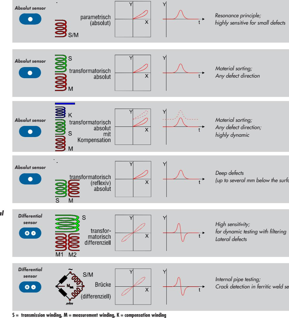
S = transmission winding, M = measurement winding, K = compensation winding
