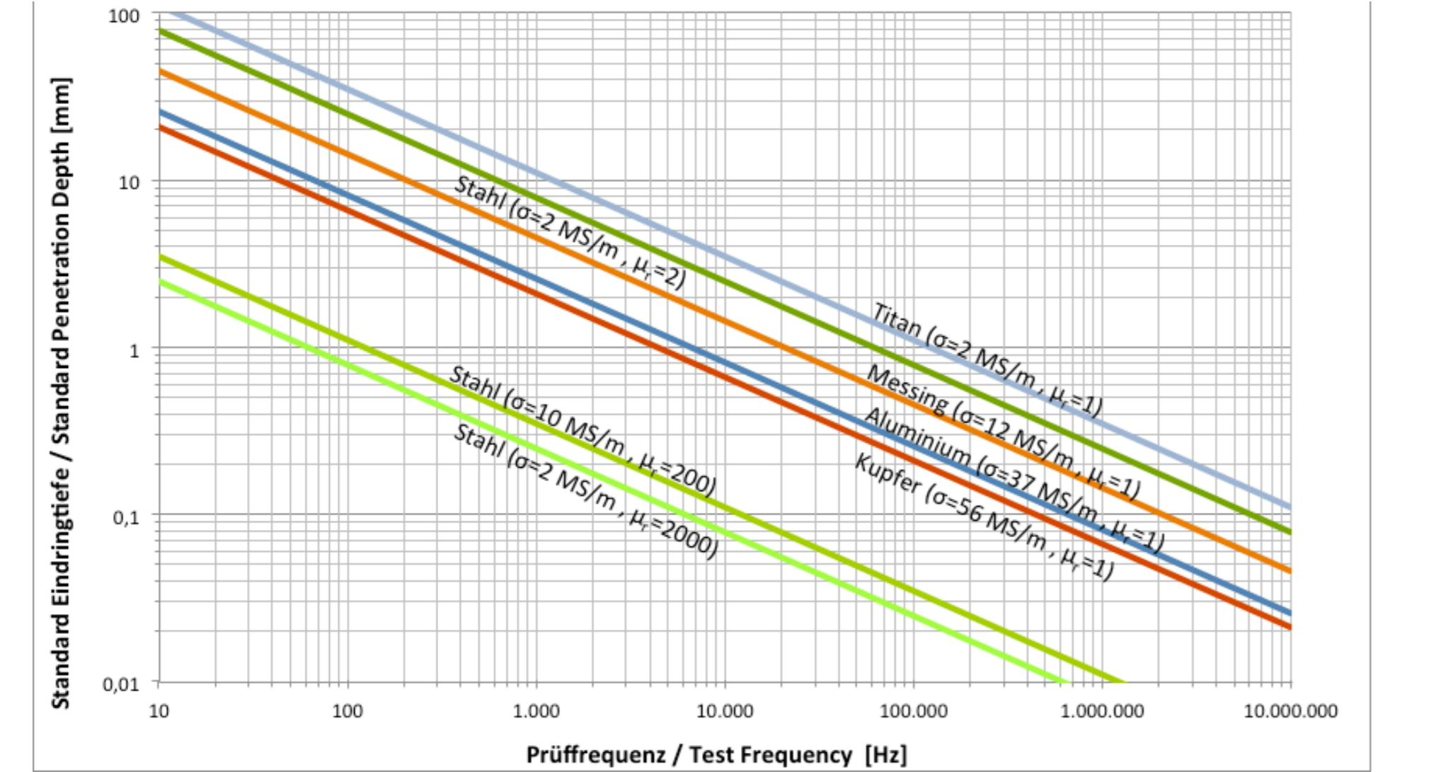
3 to 5 times the standard penetration depth. The following graph shows the standard penetration depths for different materials, depending on the test frequency. To put it simply, the selection of the test frequency influences the depth capability of the eddy current test.
