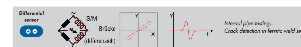
S = transmission winding, M = measurement winding, K = compensation winding
