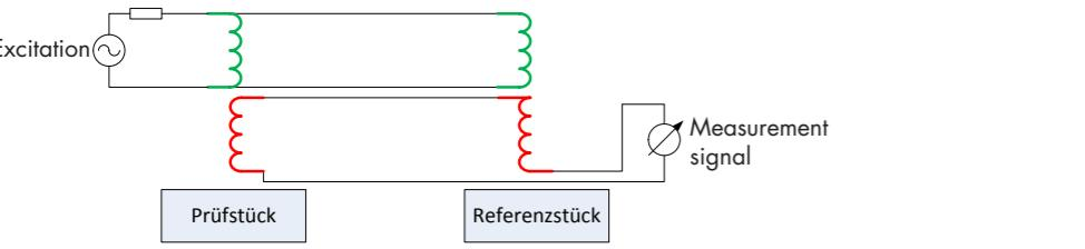
**Differential system with external comparison**
