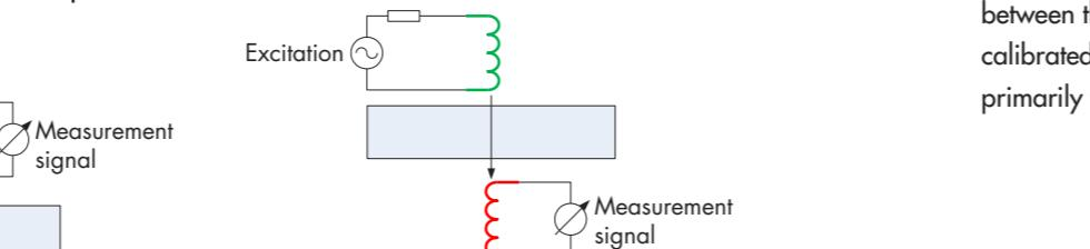
Sensors can be constructed with and without a ferrite core. However, a ferrite core concentrates and guides the magnetic sensor field.
