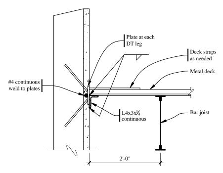
**Figure 7.3-10** Sketch of connection of non-load-bearing DT wall panel at the roof (1.0 in = 25.4 mm, 1.0 ft = 0.3048 m).
