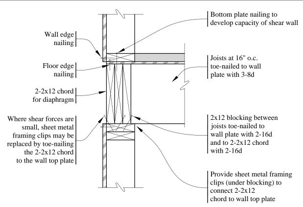
Figure 10.1-10 Bearing wall (1.0 in = 25.4 mm).
