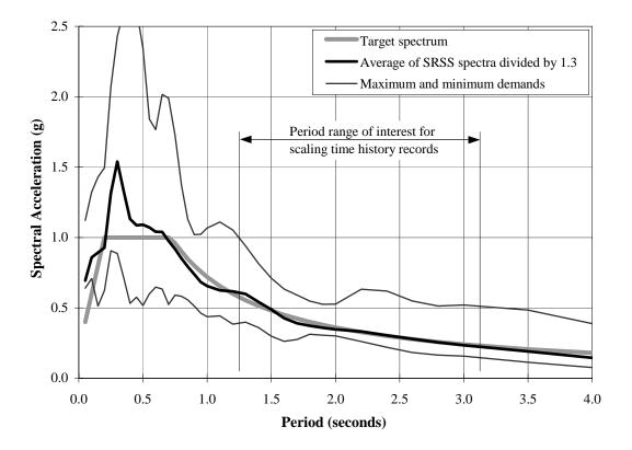
Figure 11.5-7 Comparison of design earthquake spectra.
