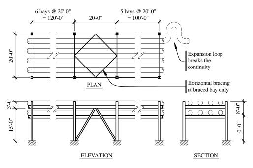
**Figure 12-2** Pipe rack (1.0 ft = 0.3048 m).
