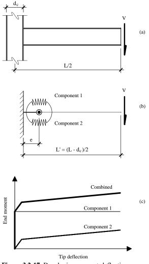
**Figure 3.2-17** Developing moment-deflection diagrams for a typical girder.
