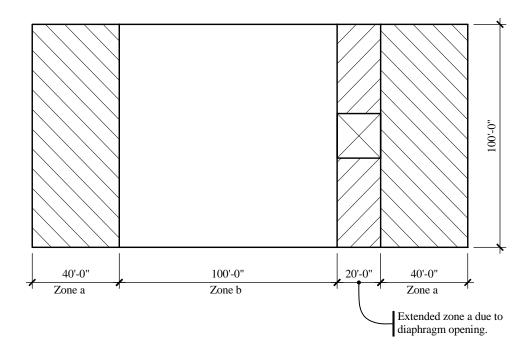
**Figure 10.2-2** Diaphragm framing and nailing layout (1.0 ft = 0.3048 m).
