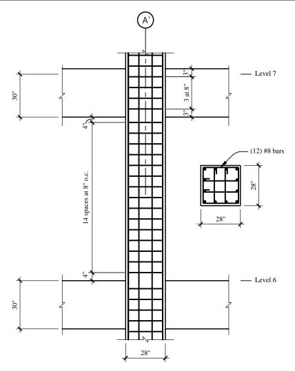
**Figure 6-45** Column reinforcement (1.0 in = 25.4 mm).
