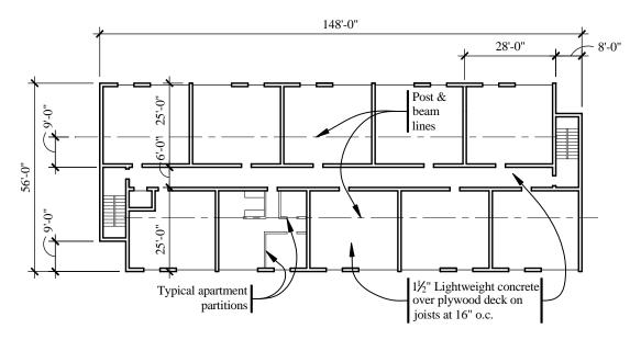
**Figure 10.1-1** Typical floor plan (1.0 ft = 0.3048 m).
