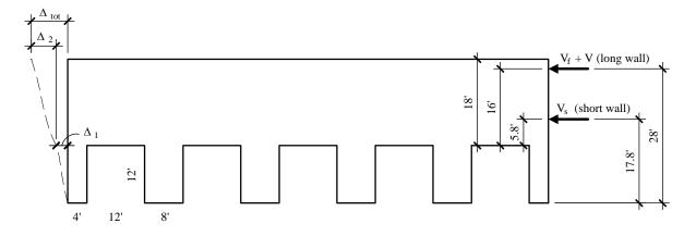
**Figure 9.1-23** In-plane deflection of end wall (1.0 ft = 0.3048 m).
