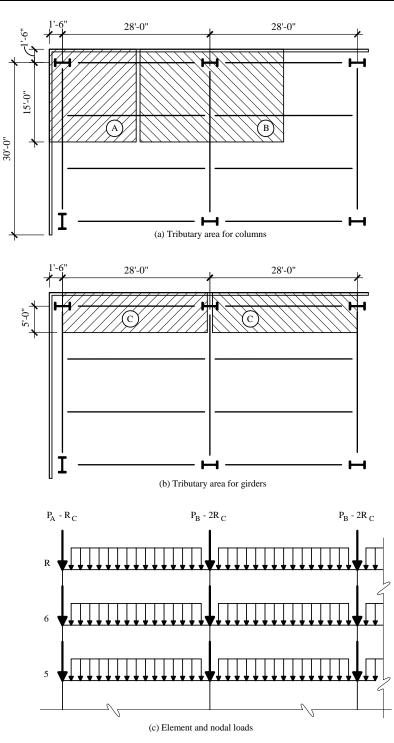
Figure 3.2-3 Element loads used in analysis.
