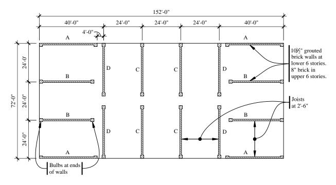
**Figure 9.3-1** Floor plan (1.0 ft = 0.3048 m, 1.0 in. = 25.4 mm)
