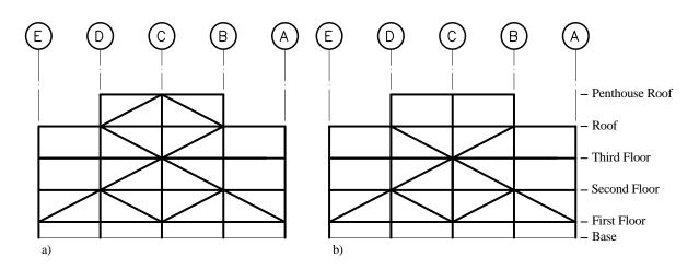
Figure 11.5-5 Transverse bracing elevations: (a) on Column Lines 2 and 6 and (b) on Column Line 4.
