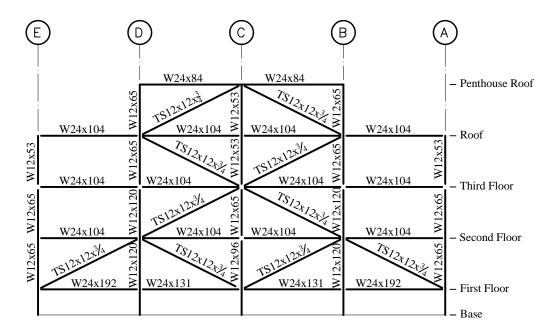
Figure 11.5-8 Elevation of framing on Column Line 2 (Column Line 6 is similar).
