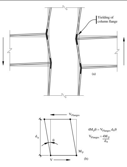
Figure 3.2-11 Column flange component of panel zone resistance.
