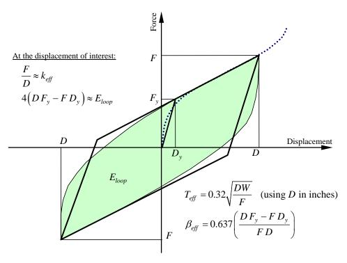
Figure 11.4-2 Bilinear idealization of isolator unit behavior.
