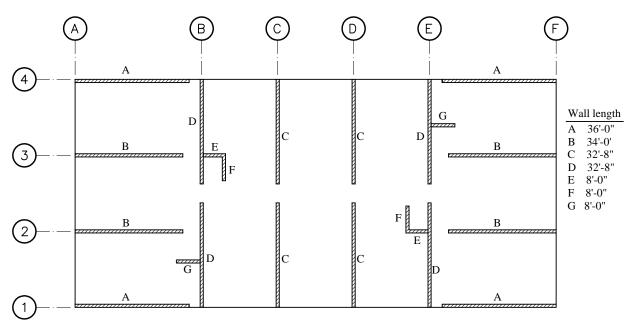
**Figure 9.2-3** Plan of walls (1.0 ft = 0.3048 m).
