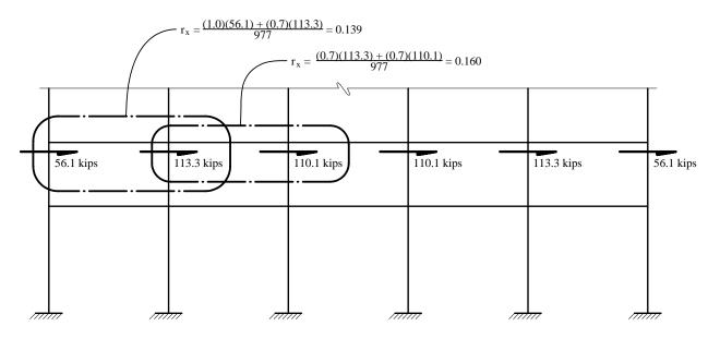
Figure 5.2-12 Column shears for N-S direction (partial elevation, Level 3) (1.0 kip = 4.45 kN).
