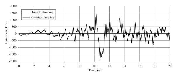
Figure 3.2-72 Base shear time histories as obtained from inertial forces (1.0 kip = 4.45 kN).
