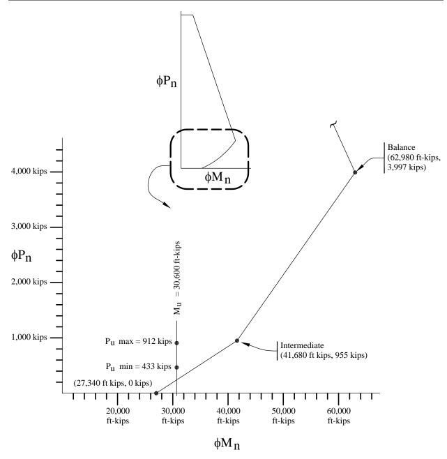
**Figure 9.3-6**  $\varphi P_{11} - \varphi M_{11}$  Diagram for Level 1 (1.0 kip = 4.45 kN, 1.0 ft-kip = 1.36 kN-m).
