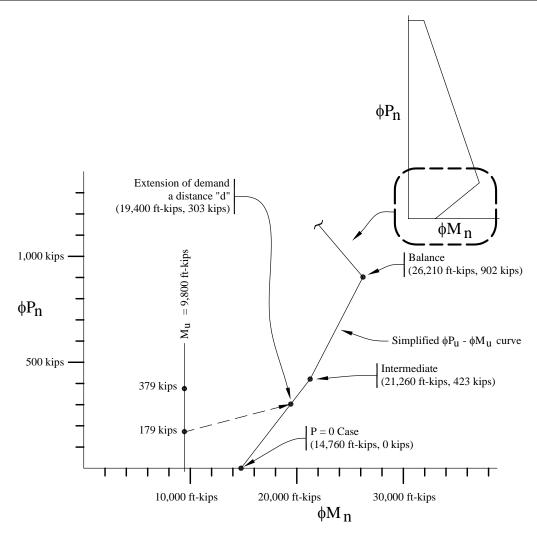
**Figure 9.3-10**  $\varphi P_{11} - \varphi M_{11}$  Diagram for Level 7 (1.0 kip = 4.45 kN, 1.0 ft-kip = 1.36 kN-m).
