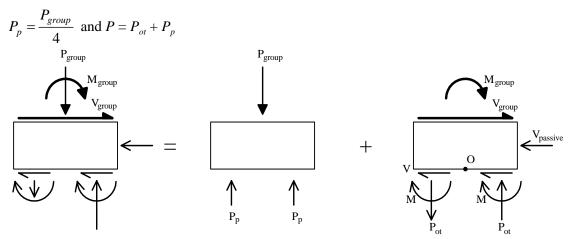
Figure 4.2-3 Pile cap free body diagram.
