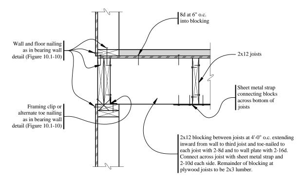
Figure 10.1-11 Nonbearing wall (1.0 in. = 25.4 mm).
