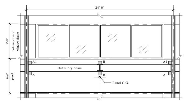
Figure 13.2-3 shows the types and locations of connections that support one spandrel panel.
