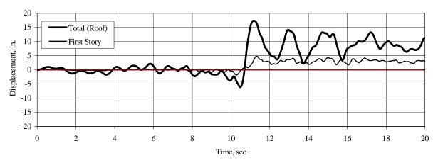
Figure 3.2-56 Time history of roof and first-story displacement, Ground Motion A00, including P-delta effects.
