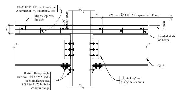
Figure 8-10 Elevation of typical connection (1.0 ft = 0.3048 m, 1.0 in. = 25.4 mm).
