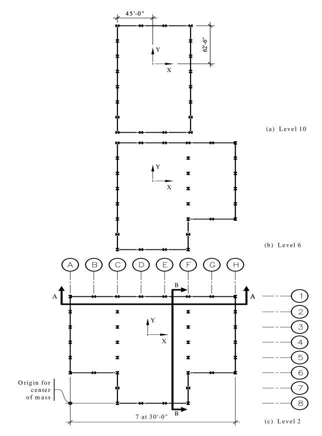
**Figure 3.1-1** Various floor plans of 12-story Stockton building (1.0 ft = 0.3048 m).
