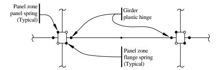
Figure 3.2-8 Model of girder and panel zone region.
