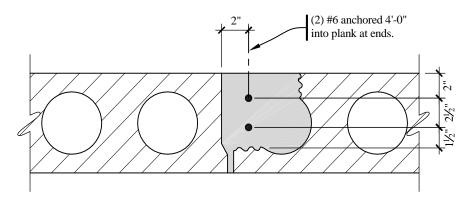
**Figure 7.1-5** Anchorage region of shear reinforcement for Joint 1 and collector reinforcement for Joint 5 (1.0 in. = 25.4 mm).
