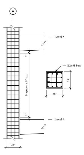
**Figure 6-50** Details for Column A, Frame 3 (1.0 in = 25.4 mm).
