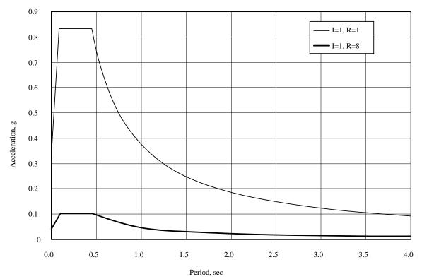
Figure 3.1-11 Total acceleration response spectrum used in analysis.
