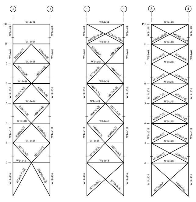
Figure 5.2-24 Braced frame of dual system in E-W-direction.
