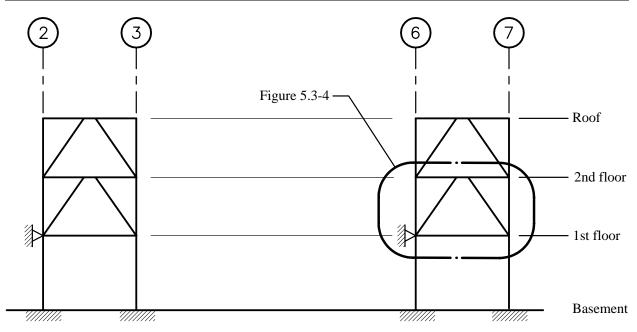
Figure 5.3-3 Diagram of eccentric braced frames on Grid F.
