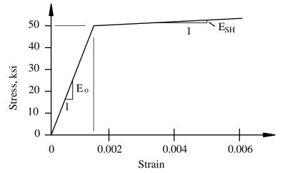
Figure 3.2-15 Assumed stress-strain curve for modeling girders.
