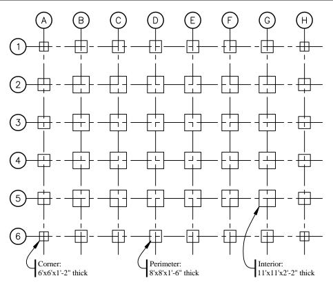
Figure 4.1-4 Foundation plan for gravity-load-resisting system.
