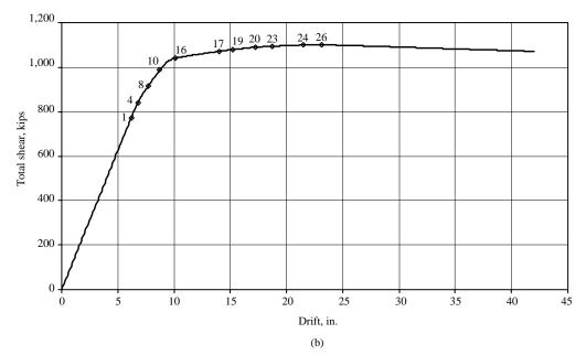
Figure 3.2-27 Patterns of plastic hinge formation: SP model under ML load, including P-delta effects.
