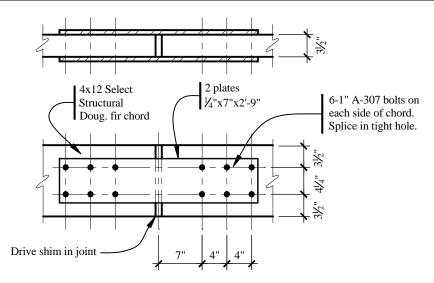
Figure 10.2-4 Chord splice detail (1.0 ft = 0.3048 m, 1.0 in. = 25.4 mm).
