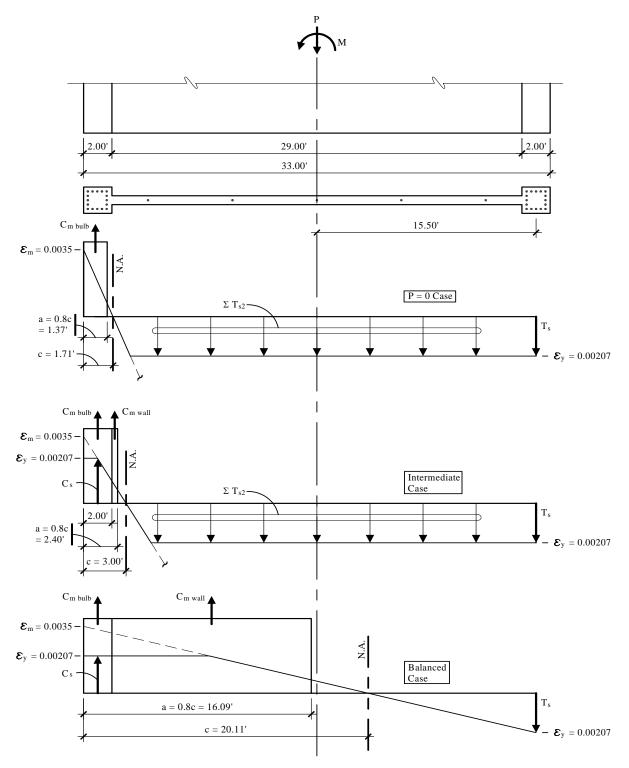
**Figure 9.3-5** Strength of Wall D, Level 1 (1.0 ft = 0.3048 m)
