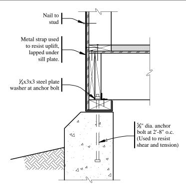
Figure 10.1-15 Perforated shear wall detail at foundation (1.0 ft = 0.3048 m, 1.0 in. = 25.4 mm).
