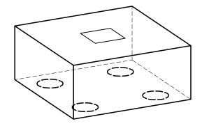
**Figure 4.2-1** Design condition: column of concrete moment resisting frame supported by pile cap and cast-in-place piles.
