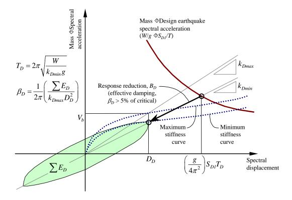
Figure 11.3-1 Isolation system capacity and earthquake demand.
