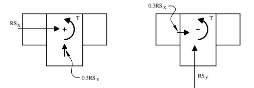
Figure 3.1-12 Load combinations from response-spectrum analysis.
