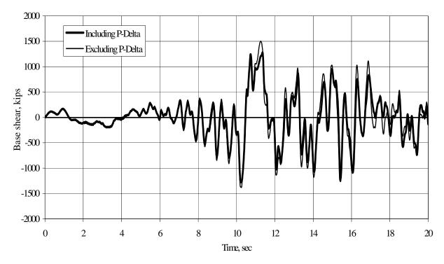
Figure 3.2-66 Time history of base shear, Ground Motion A00, with and without P-delta effects.
