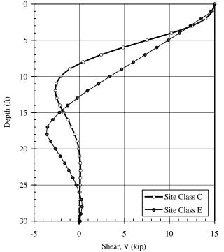
**Figure 4.2-7** Results of pile analysis – shear versus depth (applied lateral load is 15 kips).
