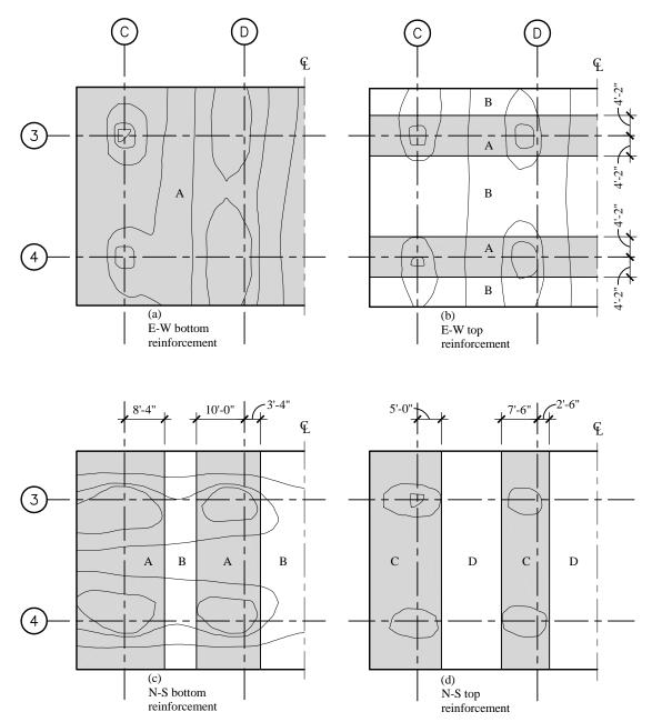
Figure 4.1-11 Mat foundation flexural reinforcement.
