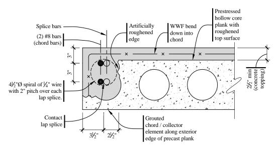
**Figure 7.1-10** Boundary member, and chord and collector reinforcement (1.0 in. = 25.4 mm).
