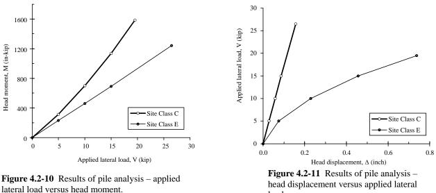
head displacement versus applied lateral load.
