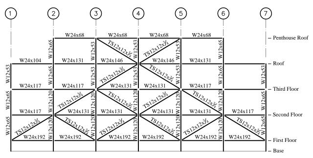
Figure 11.5-9 Elevation of framing on Column Line B (Column Line D is similar).
