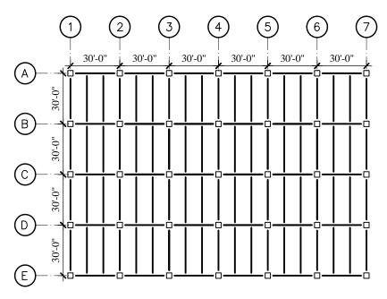
**Figure 11.5-2** Typical floor framing plan (1.0 ft = 0.3048 m).
