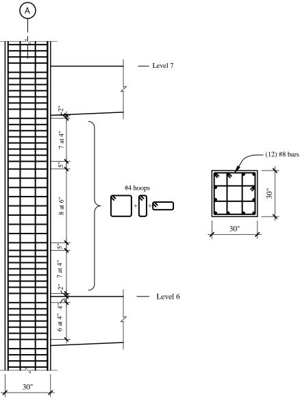
Figure 6-33 Column detail (1.0 in = 25.4 mm).
