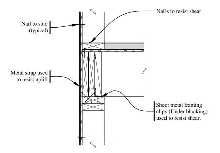
Figure 10.1-16 Perforated shear wall detail at floor framing.
