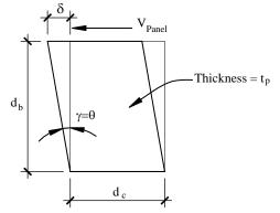
Figure 3.2-12 Column web component of panel zone resistance.
