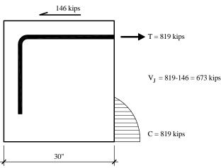
**Figure 6-30** Computing joint shear force (1.0 kip = 4.45 kN).
