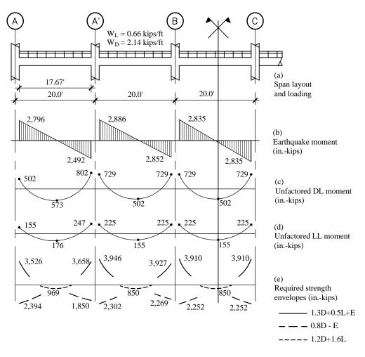
**Figure 6-40** Bending moment envelopes at Level 5 of Frame 1 (1.0 ft = 0.3048 m, 1.0 kip/ft = 14.6 kN/m, 1.0 in.-kip = 0.113 kN-m).
