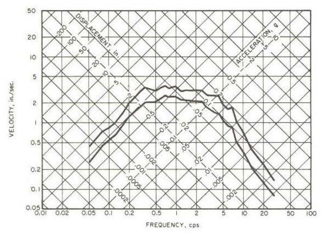
**Figure 1.2-4** Averaged spectrum (Newmark, Blume, and Kapur 1973). Mean and mean plus one standard deviation acceleration, horizontal components (2.0 percent of critical damping). Reprinted with permission from the American Society of Civil Engineers.
