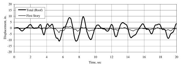
**Figure 3.2-62** Time history of roof and first-story displacement, Ground Motion C00, including P-delta effects.
