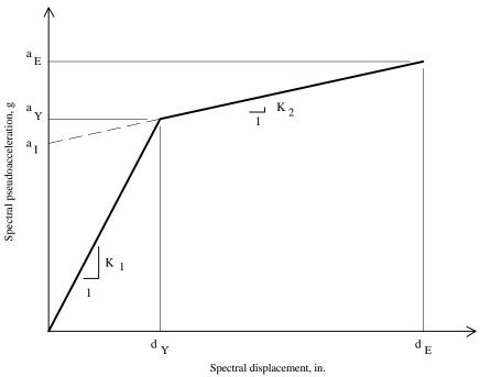
Figure 3.2-36 Capacity spectrum showing control points.
