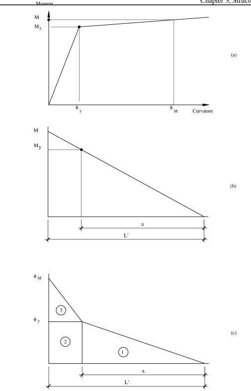
Figure 3.2-18 Development of equations for deflection of moment-deflection curves.
