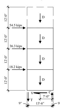
**Figure 7.2-5** Free-body diagram of the transverse walls (1.0 kip = 4.45 kN, 1.0 ft = 0.3048 m).
