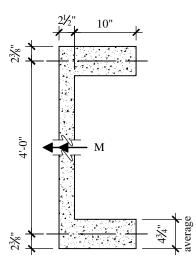
**Figure 7.3-4** Cross section of the DT dry-packed at the footing (1.0 in = 25.4 mm, 1.0 ft = 0.3048 m).
