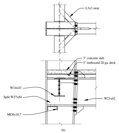
**Figure 5.1-10** Mezzanine framing (1.0 in. = 25.4 mm).
