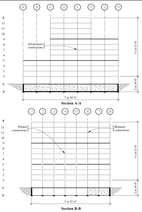
**Figure 3.1-2** Sections through Stockton building (1.0 ft. = 0.3048 m).
