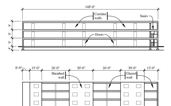
**Figure 10.1-2** Longitudinal section and elevation (1.0 ft = 0.3048 m).
