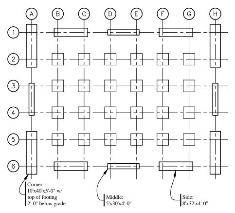
Figure 4.1-6 Foundation plan for moment-resisting frame system.
