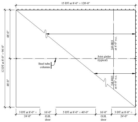
Figure 7.3-1 Single-story industrial warehouse building plan (1.0 ft = 0.3048 m).
