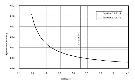
Figure 3.1-5 Computed ELF total acceleration response spectrum.
