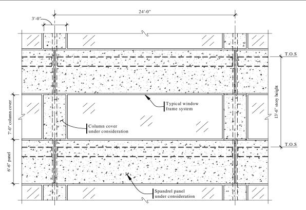
**Figure 13.2-2** Detailed building elevation (1.0 ft = 0.3048 m).
