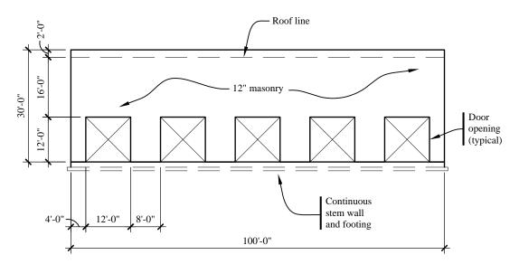
Figure 9.1-2 End wall elevation (1.0 in = 25.4 mm, 1.0 ft = 0.3048 m).
