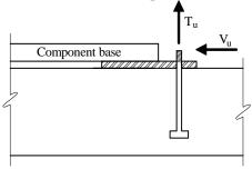
Figure 13.3-3 Anchor for direct attachment to structure.
