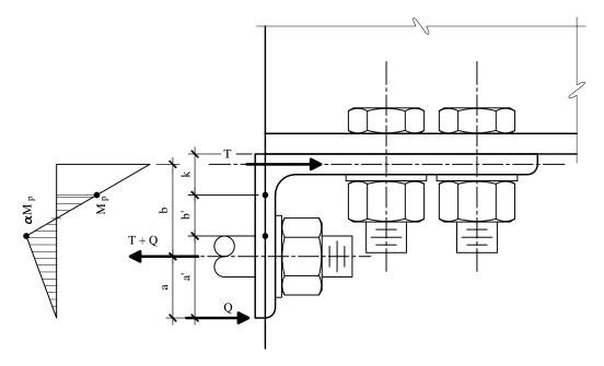
Figure 8-7 Analysis of seat angle for tension.
