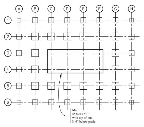
Figure 4.1-9 Foundation plan for concentrically braced frame system.
