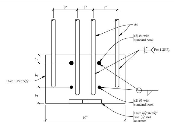
Figure 7.3-9 Details of the embedded plate in the DT at the base (1.0 in = 25.4 mm).
