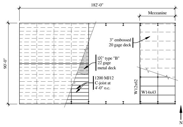
Figure 5.1-2 Roof framing and mezzanine framing plan (1.0 in. = 25.4 mm, 1.0 ft = 0.3048 m).
