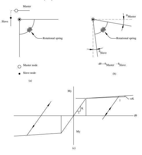
Figure 3.2-9 A compound node and attached spring.
