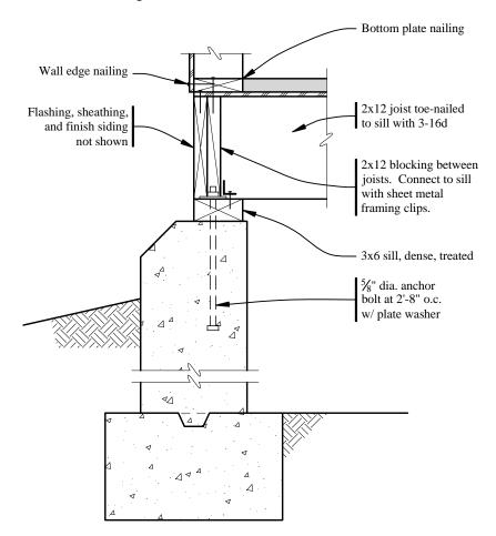
**Figure 10.1-12** Foundation wall detail (1.0 in. = 25.4 mm).
