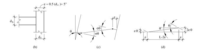
Figure 3.2-6 Plastic mechanism for computing lateral strength.
