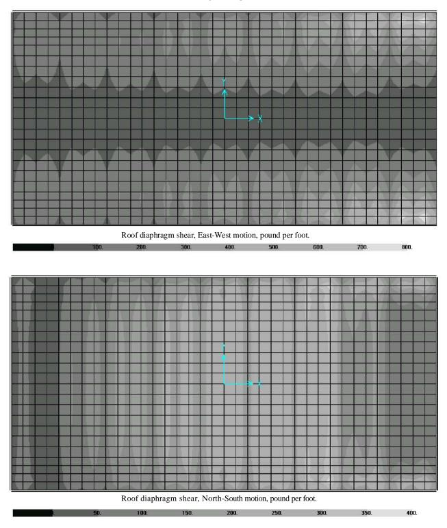
**Figure 5.1-11** Shear force in roof deck diaphragm; upper diagram is for E-W motion and lower is for N-S motion (1.0 lb. /ft. = 14.59 N/M).
