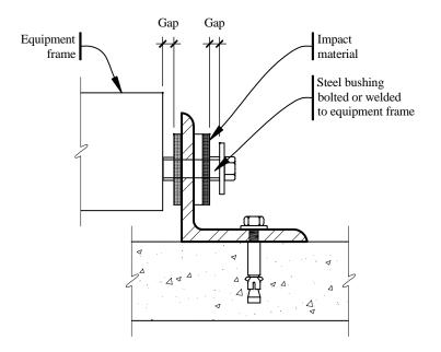
Figure 13.3-6 Lateral restraint required to resist seismic forces.
