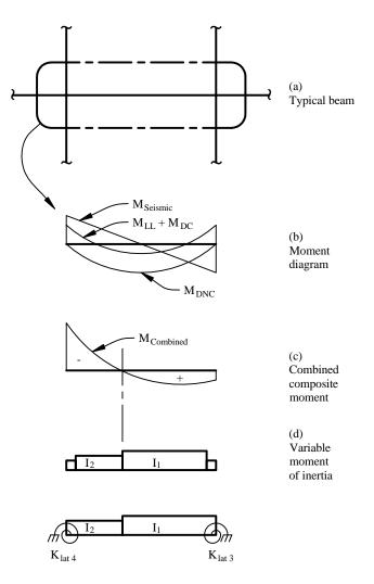
Figure 8-8 Moment diagram for typical beam.
