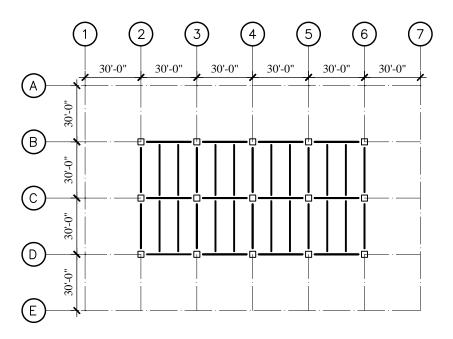
**Figure 11.5-3** Penthouse roof framing plan (1.0 ft = 0.3048 m).
