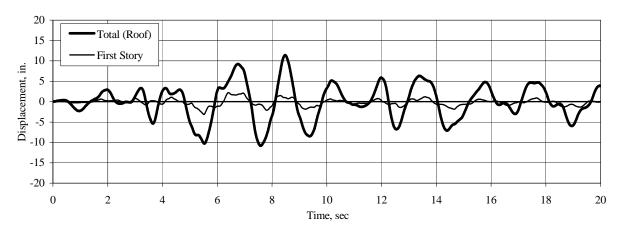
Figure 3.2-53 Time history of roof and first-story displacement, Ground Motion C00, excluding P-delta effects.
