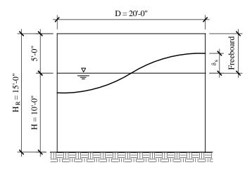
**Figure 12-6** Storage tank section (1.0 ft = 0.3048 m).
