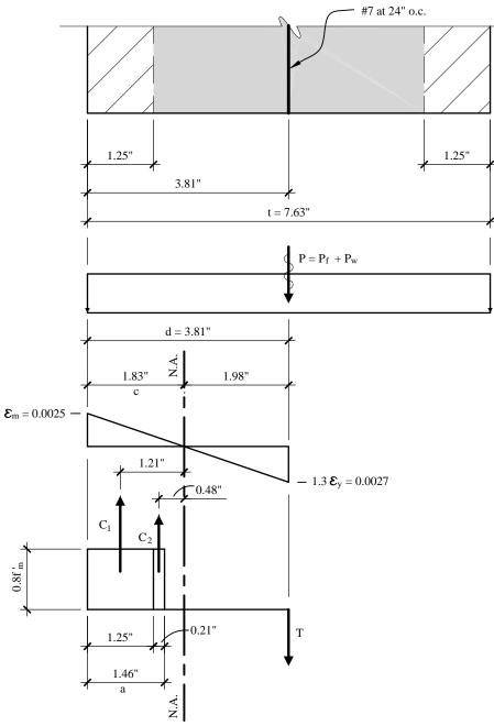
**Figure 9.1-4** Investigation of out-of-plane ductility for the 8-in.-thick CMU side walls (1.0 in = 25.4 mm).
