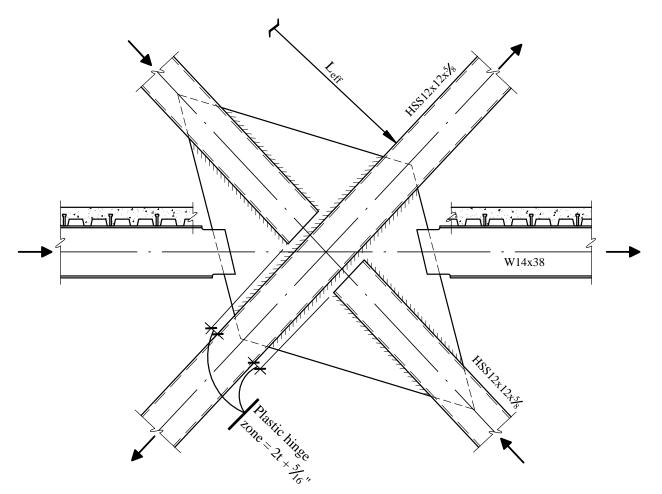
Figure 5.2-21 Brace-to-brace connection (1.0 in. = 25.4 mm).
