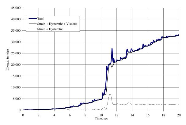
Figure 3.2-73 Energy time-history for structure with discrete added damping (1.0 in.-kip = 0.113 kN-m).
