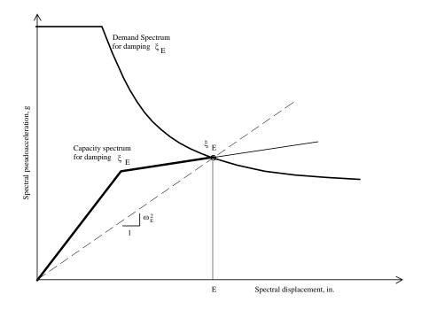
Figure 3.2-35 Capacity and demand spectra plotted together.
