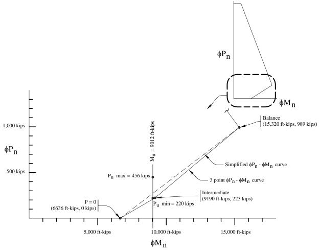
**Figure 9.2-14**  $\varphi P_{11} - \varphi M_{11}$  diagram for Los Angeles Wall D (1.0 kip = 4.45 kN, 1.0 kip-ft = 1.36 kN-m).
