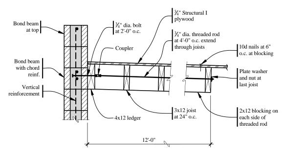
Figure 10.2-12 Anchorage of masonry wall parallel to joists (1.0 ft = 0.3048 m, 1.0 in. = 25.4 mm)
