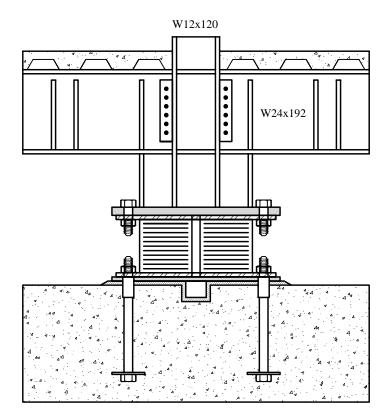
Figure 11.5-11 Typical detail of the isolation system at columns (for clarity, some elements not shown).
