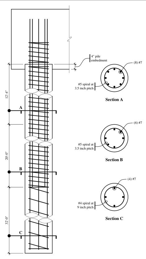
Figure 4.2-17 Pile detailing for Site Class E (under corner column).
