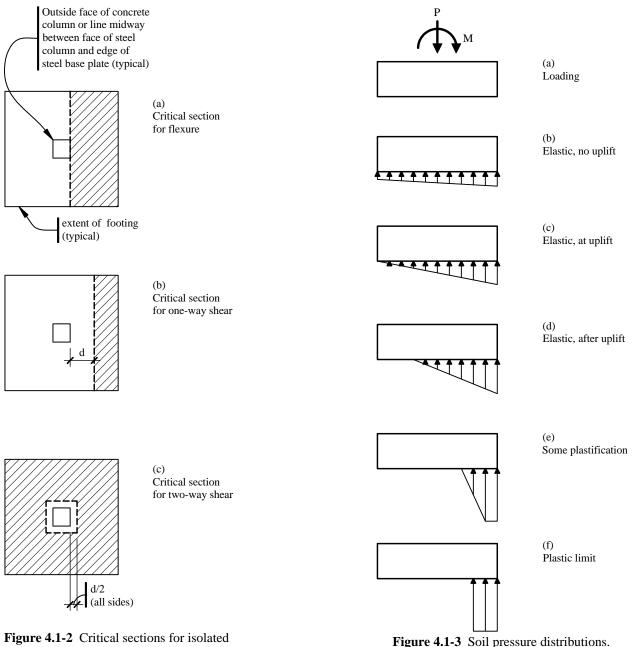
Figure 4.1-2 Critical sections for isolated footings.
