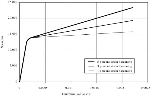
Figure 3.2-16 Moment curvature diagram for W27x94 girder.
