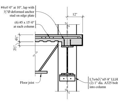
Figure 8-14 Detail at spandrel.
