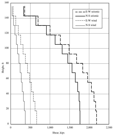
**Figure 6-3** Comparison of wind and seismic story shears for the Berkeley building (1.0 ft = 0.3048 m, 1.0 kip = 4.45 kN).
