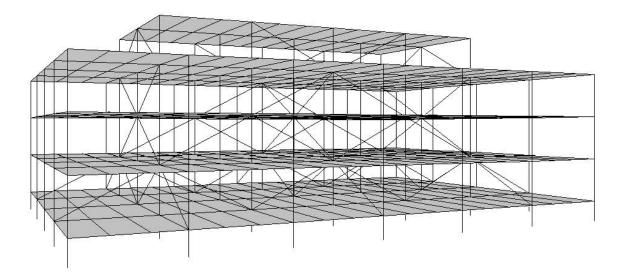
Figure 11.5-1 Three-dimensional model of the structural system.
