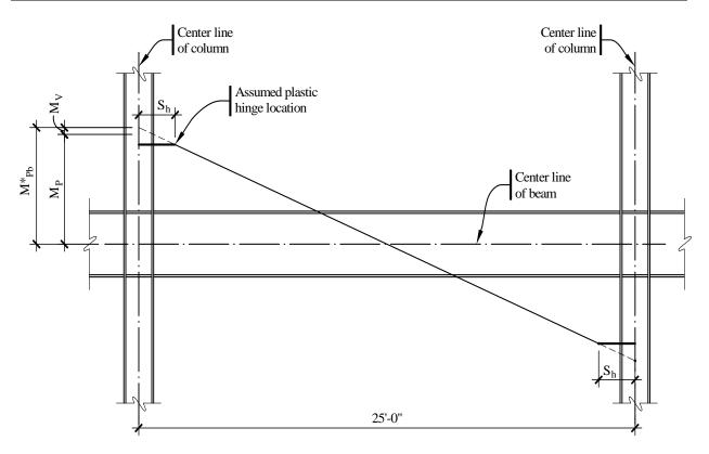
Figure 5.2-7 Projection of expected moment strength of beam (1.0 in = 25.4 mm, 1.0 ft = 0.3048 m).
