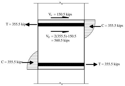
Figure 6-17 Computing joint shear stress (1.0 kip = 4.45kN).
