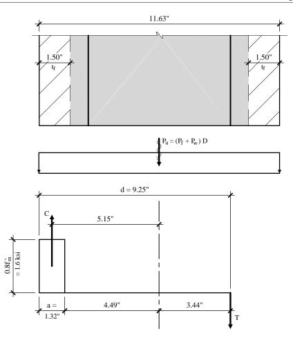
**Figure 9.1-16** Out-of-plane seismic strength of pier on end wall (1.0 in = 25.4 mm, 1.0 ksi = 6.89 MPa).
