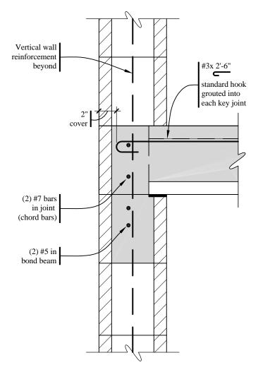
**Figure 7.1-7** Joint 4 exterior longitudinal walls to diaphragm reinforcement and out-of-plane anchorage (1.0 in. = 25.4 mm, 1.0 ft = 0.3048 m).
