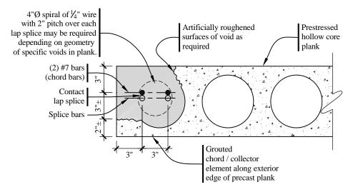
Figure 7.1-3 Joint 3 chord reinforcement at the exterior edge (1.0 in. = 25.4 mm).
