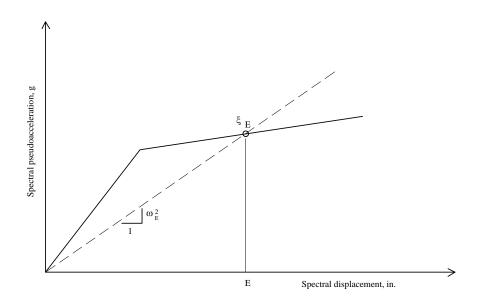
Figure 3.2-33 A simple capacity spectrum.
