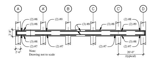
Figure 6-15 Preliminary rebar layout for Frame 1 (1.0 ft = 03.048 m).
