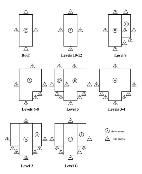
Figure 3.1-4 Key diagram for computation of floor mass.
