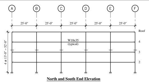
**Figure 8-2** Building end elevation (1.0 ft = 0.3048 m).
