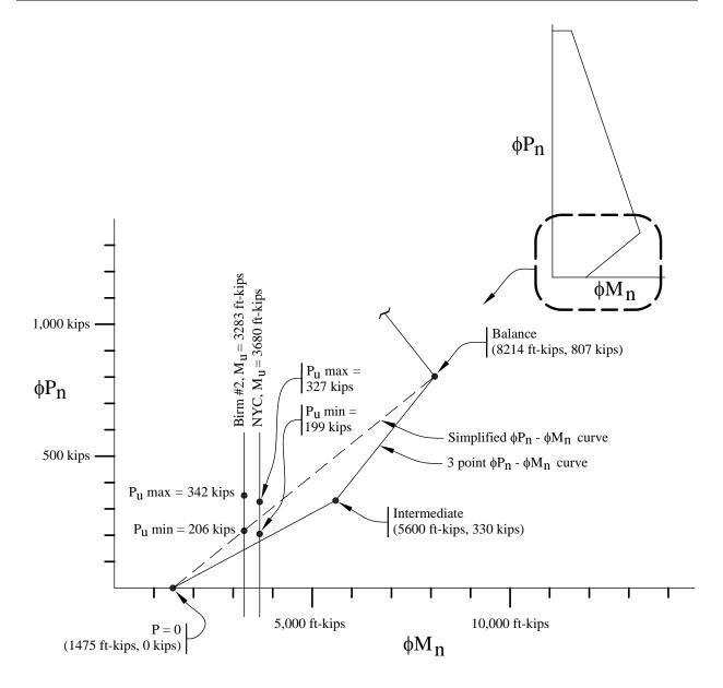
**Figure 9.2-10**  $\varphi P_{11} - \varphi M_{11}$  Diagram for New York City and Birmingham 2 Wall D (1.0 kip = 4.45 kN, 1.0 ft-kip = 1.36 kN-m).
