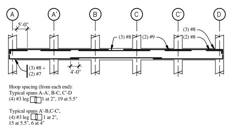
Figure 6-21 Final bar arrangement (1.0 ft = 0.3048 m, 1.0 in = 25.4 mm).
