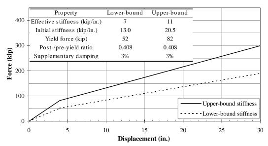
**Figure 11.5-12** Stiffness and damping properties of EOC isolator units (1.0 in. = 25.4 mm, 1.0 kip = 4.45 kN).
