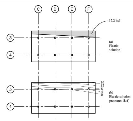
Figure 4.1-8 Soil pressures for controlling bidirectional case.
