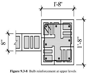
Figure 9.3-8 Bulb reinforcement at upper levels (1.0 ft = 0.3048 m, 1.0 in. = 25.4 mm).
