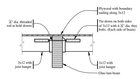
**Figure 10.2-10** Chord tie at roof opening (1.0 in. = 25.4 mm).
