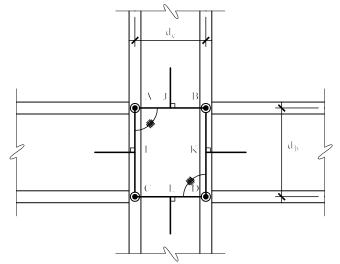
Figure 3.2-10 Krawinkler beam-column joint model.
