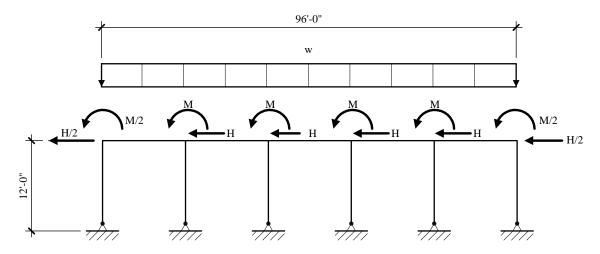
Figure 9.1-17 Input loads for in-plane end wall analysis (1.0 ft = 0.3048 m).
