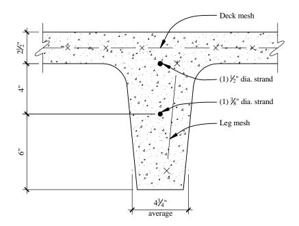
**Figure 7.3-5** Cross section of one DT leg showing the location of the bonded prestressing tendons or strand (1.0 in = 25.4 mm).
