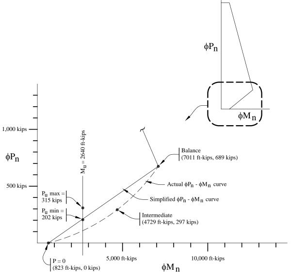
**Figure 9.2-6**  $\varphi P_{11} - \varphi M_{11}$  diagram for Birmingham 1 Wall D (1.0 kip = 4.45 kN, 1.0 ft-kip = 1.36 kN-m).
