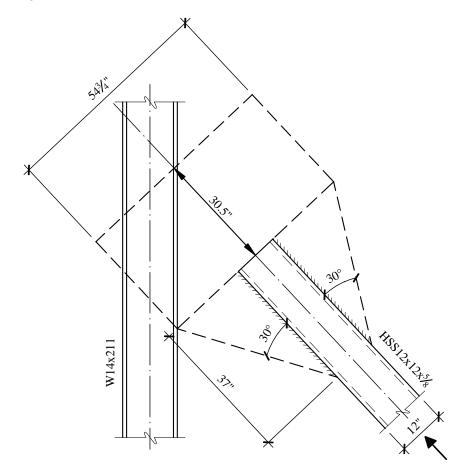
Figure 5.2-20 Whitmore section (1.0 in. = 25.4 mm, 1.0 ft = 0.3048 m).
