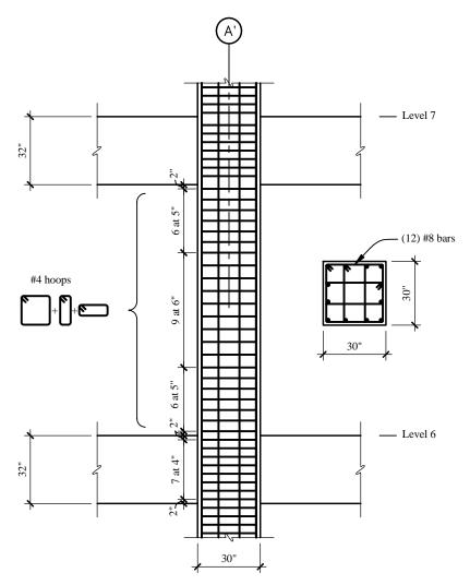
**Figure 6-26** Details of reinforcement for column (1.0 in = 25.4 mm).
