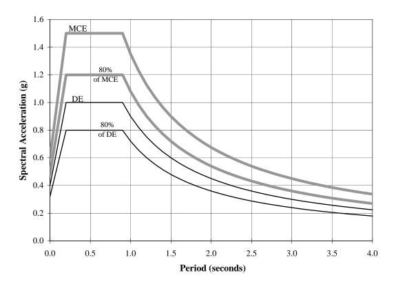
Figure 11.5-6 Example design spectra (5 percent damping).
