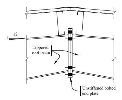
Figure 5.1-9 End plate connection at ridge.
