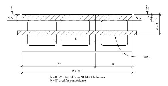
**Figure 9.1-7** Cracked moment of inertia  $(I_{cr})$  for 8-in.-thick CMU side walls (1.0 in = 25.4 mm).
