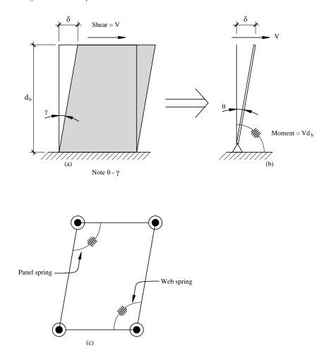
**Figure 3.2-14** Transforming shear deformation to rotational deformation in the Krawinkler model.
