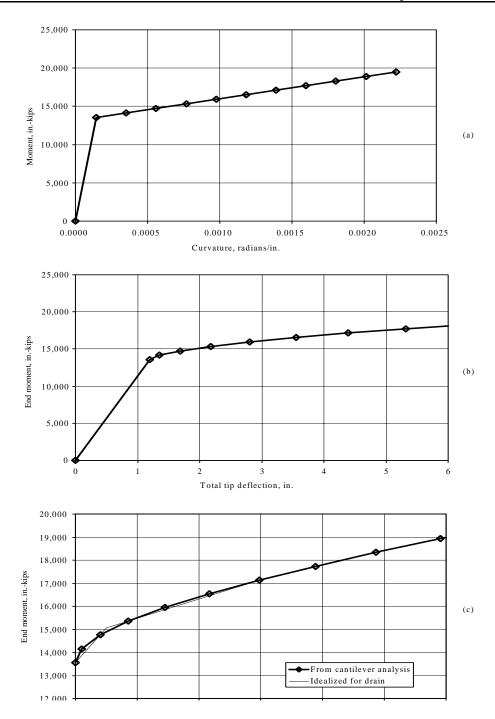
**Figure 3.2-19** Moment-deflection curve for W27x94 girder with 3 percent strain hardening.
