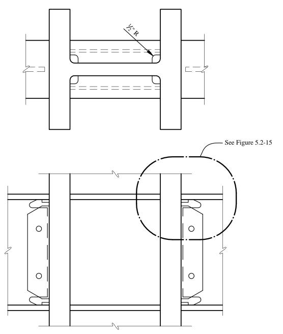
Figure 5.2-14 WUF-W connection, Second level, NS-direction (1.0 in. = 25.4 mm).
