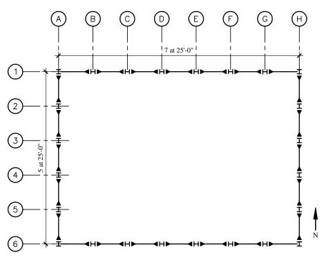
Figure 4.1-5 Framing plan for moment resisting frame system.
