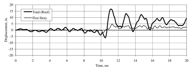
**Figure 3.2-47** Time history of roof and first-story displacement, Ground Motion A00, excluding P-delta effects.
