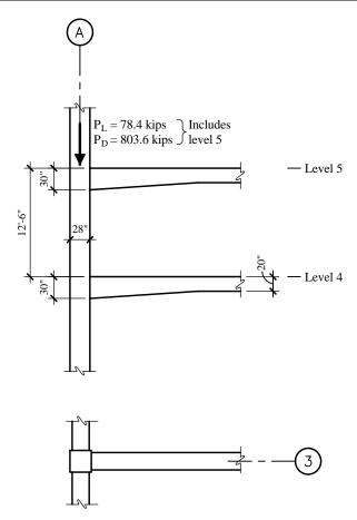
**Figure 6-48** Loading for Column A, Frame 3 (1.0 ft = 0.3048 m, 1.0 in = 25.4 mm, 1.0 kip = 4.45kN).
