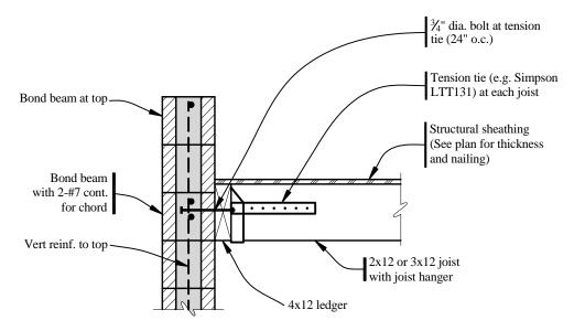
Figure 10.2-9 Anchorage of masonry wall perpendicular to joists (1.0 in. = 25.4 mm).
