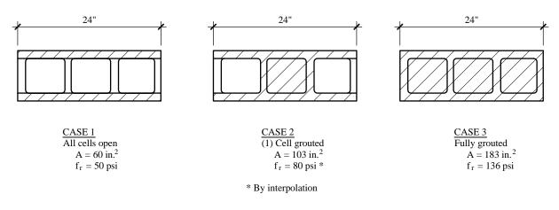
Figure 9.1-6 Basis for interpolation of modulus of rupture,  $f_r$  (1.0 in = 25.4 mm, 1.0 psi = 6.89 kPa).
