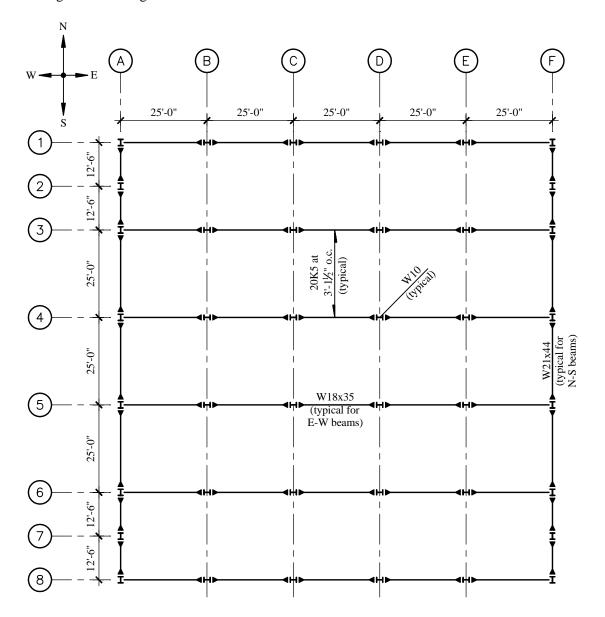
**Figure 8-1** Typical floor plan (1.0 ft = 0.3048 m).
