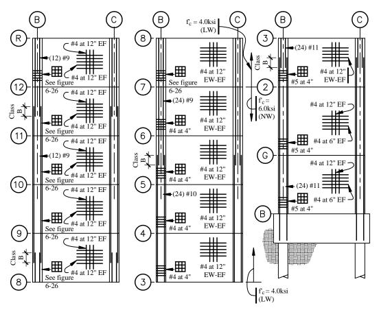
Figure 6-37 Overall details of structural wall (1.0 in = 25.4 mm).
