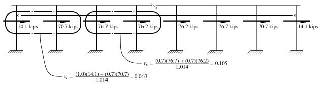
Figure 5.2-11 Column shears for E-W direction (partial elevation, Level 2) (1.0 kip = 4.45 kN).
