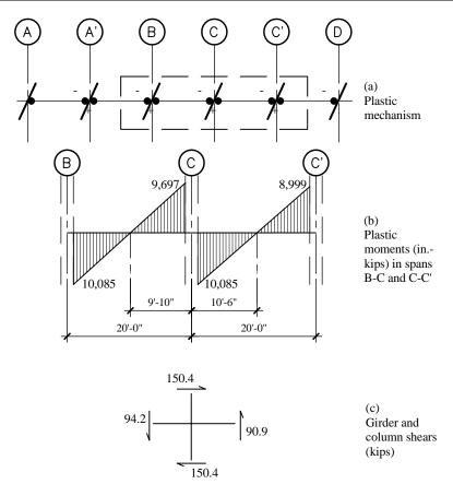
**Figure 6-16** Diagram for computing column shears (1.0 ft = 0.3048 m, 1.0 kip = 4.45 kN, 1.0 in.-kip = 0.113 kN-m).
