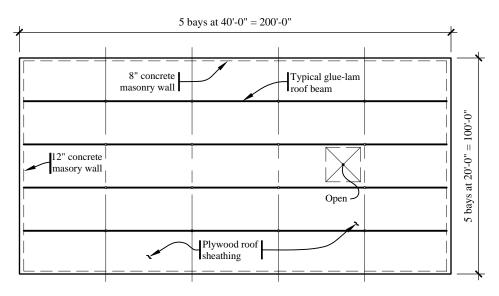
**Figure 9.1-1** Roof plan (1.0 in = 25.4 mm, 1.0 ft = 0.3048 m).
