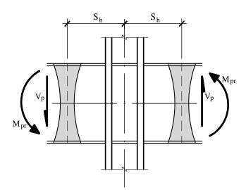
Figure 5.2-13 Forces at beam/column connection.
