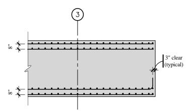
Figure 4.1-12 Section of mat foundation.
