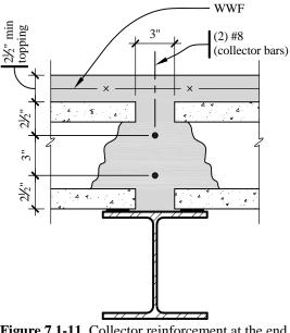
**Figure 7.1-11** Collector reinforcement at the end of the interior longitudinal walls - Joint 5 (1.0 in. = 25.4 mm, 1.0 ft = 0.3048 m).
