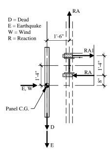
Figure 13.2-5 Spandrel panel connection forces.
