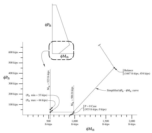
**Figure 9.1-21** In-plane  $\varphi P_{11} - \varphi M_{11}$  diagram for pier (1.0 kip = 4.45 kN, 1.0 ft-kip = 1.36 kN-m).
