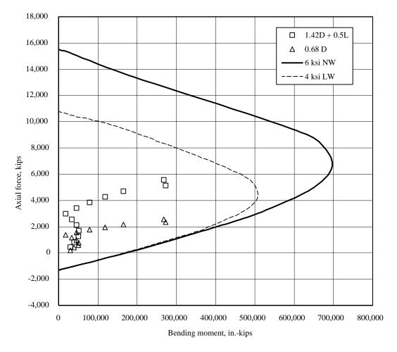
Figure 6-34 Interaction diagram for structural wall (1.0 kip = 4.45kN, 1.0 in.-kip = 0.113 kN-m).
