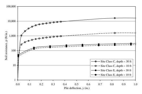
**Figure 4.2-4** Representative *p*-*y* curves (note that a logarithmic scale is used on the vertical axis).
