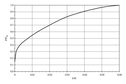
Figure 4.2-5 Passive pressure mobilization curve (after FEMA 356).
