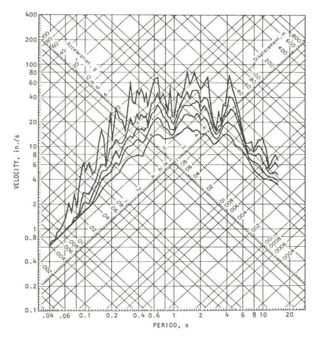
**Figure 1.2-3** Response spectrum of north-south ground acceleration (0, 0.02, 0.05, 0.10, 0.20 of critical damping) recorded at the Holiday Inn, approximately 5 miles from the causative fault in the 1971 San Fernando earthquake (Housner and Jennings 1982).
