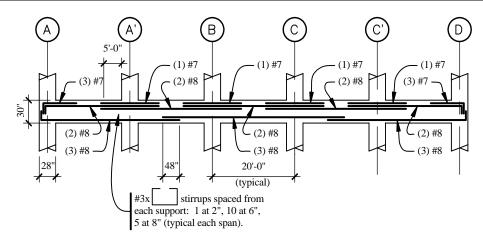
**Figure 6-41** Preliminary reinforcement layout for Level 5 of Frame 1 (1.0 in = 25.4 mm, 1.0 ft = 0.3048 m).
