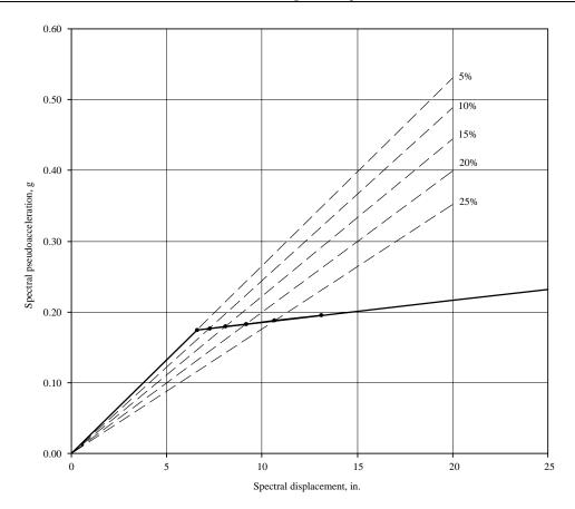
Figure 3.2-39 Capacity spectrum with equivalent viscous damping points and secant stiffnesses.
