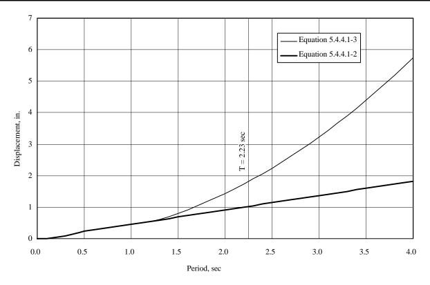
Figure 3.1-6 Computed ELF relative displacement response spectrum (1.0 in. = 25.4 mm).
