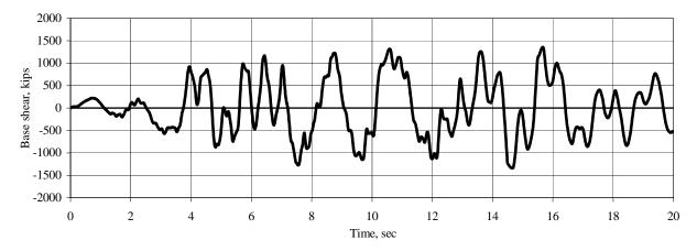
Figure 3.2-60 Time history of total base shear, Ground Motion B00, including P-delta effects.
