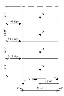
**Figure 7.2-4** Free-body diagram for longitudinal walls (1.0 kip = 4.45 kN, 1.0 ft = 0.3048 m).
