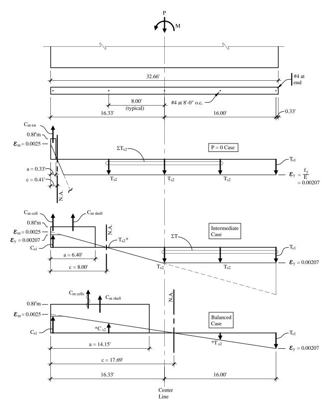
**Figure 9.2-5** Strength of Birmingham 1 Wall D (1.0 ft = 0.3048 m). Strain diagram superimposed on strength diagram for the three cases. The low force in the reinforcement is neglected in the calculations.
