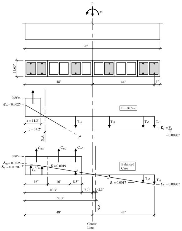
**Figure 9.1-20** In-plane seismic strength of pier (1.0 in = 25.4 mm). Strain diagram superimposed on strength diagram for both cases. Note that low force in reinforcement is neglected in calculations.
