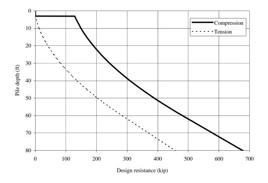
Figure 4.2-14 Pile axial capacity as a function of length for Site Class C.
