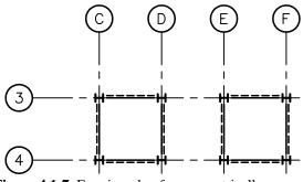
**Figure 4.1-7** Framing plan for concentrically braced frame system.
