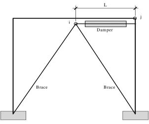
Figure 3.2-69 Modeling a simple damper.
