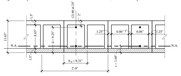
**Figure 9.1-15** Cracked moment of inertia ( $I_{cr}$ ) for end walls (1.0 in = 25.4 mm, 1.0 ft = 0.3048 m). Dimension "c" depends on calculations shown for Figure 9.1-16.
