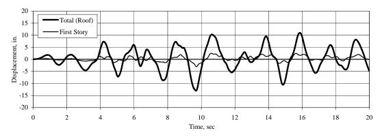
**Figure 3.2-50** Time history of roof and first-story displacement. Ground Motion B00, excluding P-delta effects.
