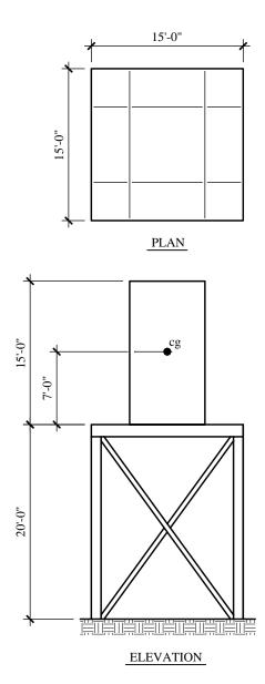
Figure 12-7 Platform for elevated transformer (1.0 ft = 0.3048 m).
