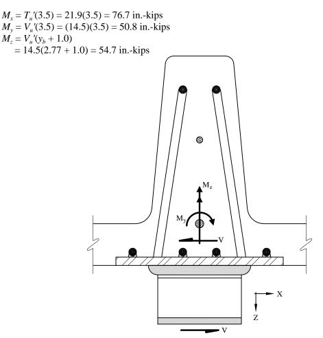
**Figure 7.3-7** Free-body of angle with welds, top view, showing only shear forces and resisting moments.
