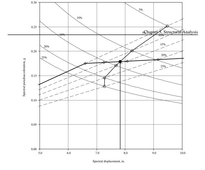
Figure 3.2-42 Close-up view of portion of capacity and demand spectra.
