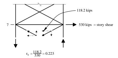
**Figure 5.2-18** Lateral force component in braces for N-S direction – partial elevation, Level 7 (1.0 kip = 4.45 kN).
