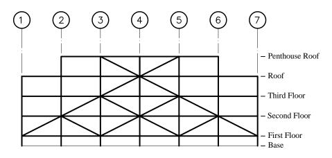
Figure 11.5-4 Longitudinal bracing elevation (Column Lines B and D).
