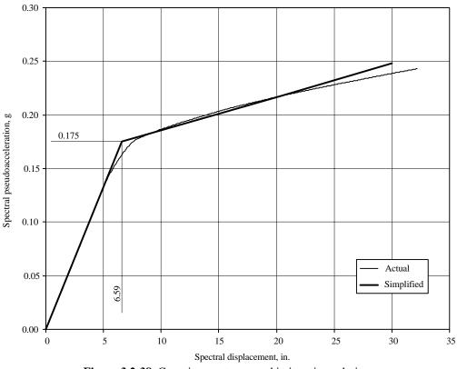
Figure 3.2-38 Capacity spectrum used in iterative solution.
