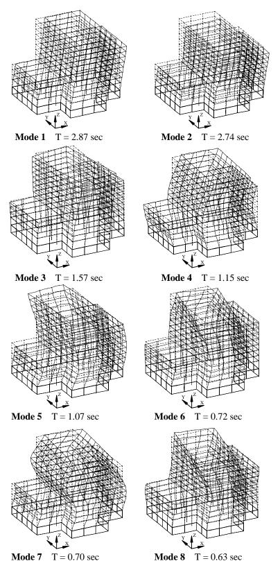
Figure 3.1-10 Mode shapes as computed using SAP2000.
