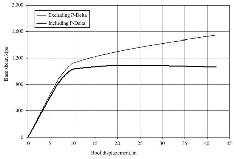
Figure 3.2-25 Response of strong panel model to ML loads, with and wthout P-delta effects.
