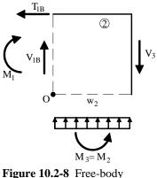
Figure 10.2-8 Free-body diagram for Element 2.
