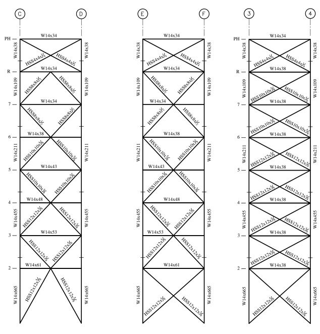
Figure 5.2-16 Braced frame in E-W direction.
