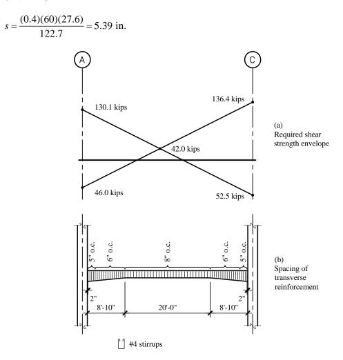
**Figure 6-47** Shear force envelope for haunched girder (1.0 ft = 0.3048m, 1.0 in = 25.4 mm, 1.0 kip = 4.45kN).
