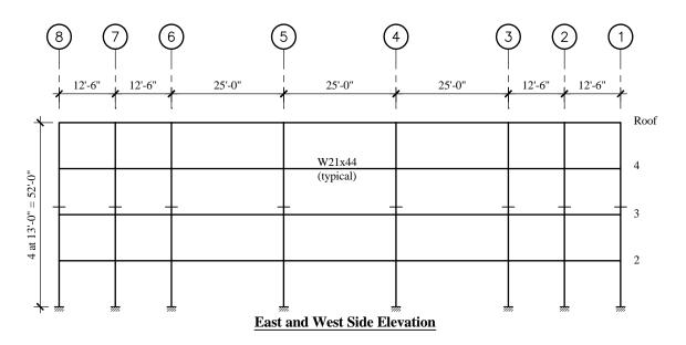
**Figure 8-3** Building side elevation (1.0 ft = 0.3048 m).
