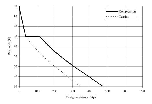
Figure 4.2-15 Pile axial capacity as a function of length for Site Class E.
