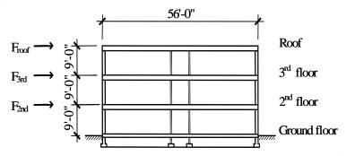
**Figure 10.1-5** Vertical shear distribution (1.0 ft = 0.3048 m).
