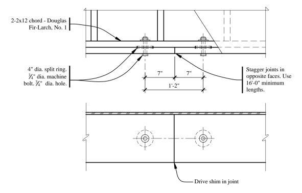
Figure 10.1-13 Diaphragm chord splice (1.0 ft = 0.3048 m, 1.0 in. = 25.4 mm).
