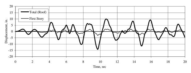
Figure 3.2-59 Time history of roof and first-story displacement, Ground Motion B00, including P-delta effects.
