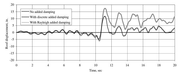
decrease in roof displacement. It is also clear that the discrete dampers and the equivalent Rayleigh damping produce very similar results.
