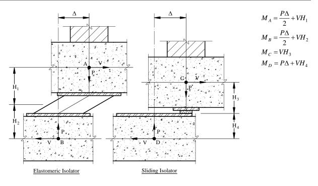
Figure 11.4-1 Moments due to horizontal shear and P-delta effects.
