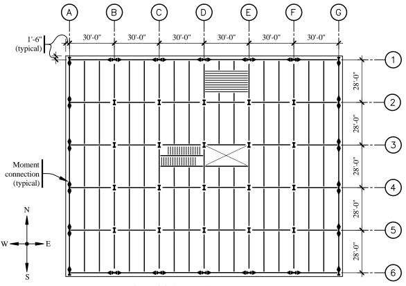
Figure 3.2-1 Plan of structural system.
