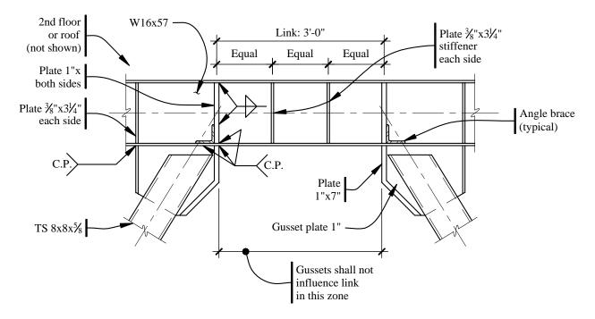
Figure 5.3-5 Link and upper brace connection (1.0 in. = 25.4 mm, 1.0 ft = 0.3048 m).
