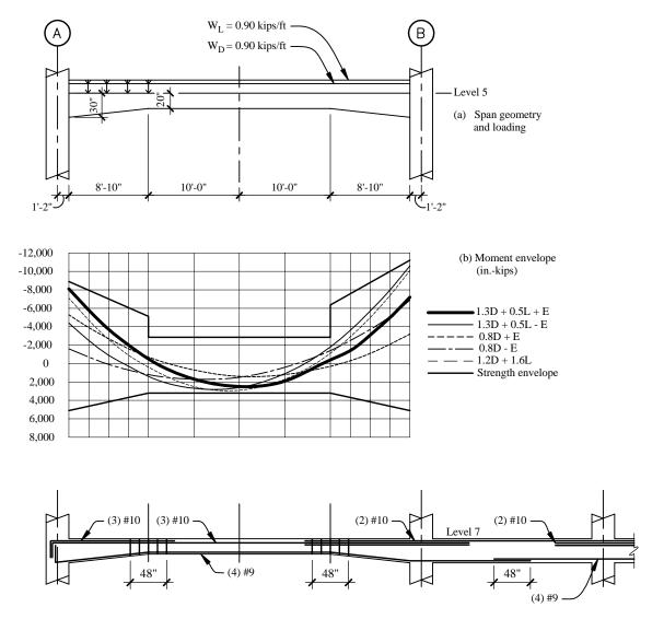
**Figure 6-46** Loads, moments, and reinforcement for haunched girder (1.0 in = 25.4 mm, 1.0 ft = 0.3048 m, 1.0 kip/ft = 14.6 kN/m, 1.0 in.-kip = 0.113 kN-m).
