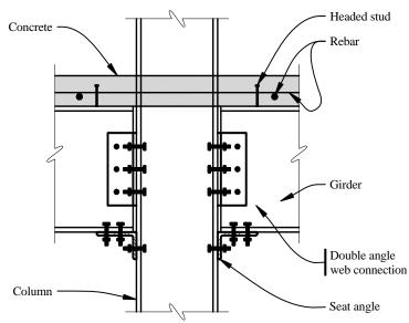
Figure 8-4 Typical composite connection.
