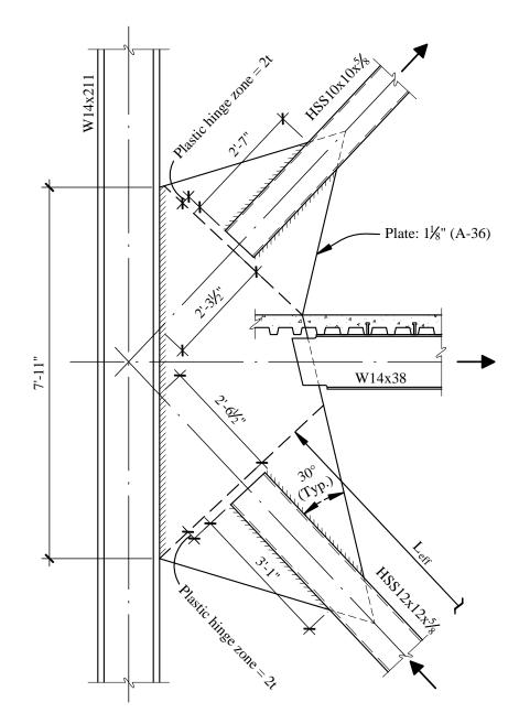
**Figure 5.2-19** Bracing connection detail (1.0 in. = 25.4 mm, 1.0 ft = 0.3048 m).
