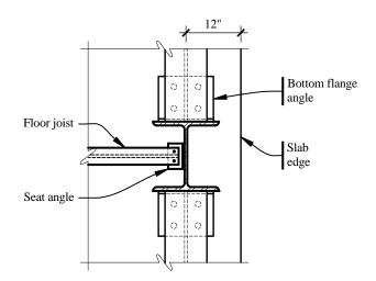
Figure 8-13 Detail at column.
