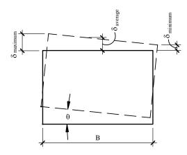
**Figure 3.1-7** Amplification of accidental torsion.
