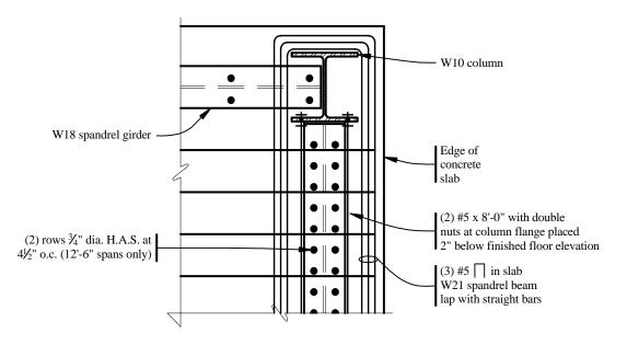
Figure 8-15 Detail at building corner.
