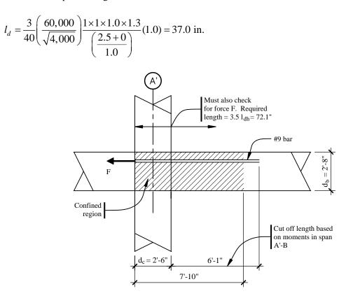
Figure 6-20 Development length for top bars (1.0 ft = 0.3048 m, 1.0 in = 25.4 mm).
