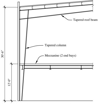
**Figure 5.1-6** Gable frame schematic: Column tapers from 12 in. at base to 36 in. at knee; roof beam tapers from 36 in. at knee to 18 in. at ridge; plate sizes are given in Figure 5.1-8 (1.0 in. = 25.4 + mm).
