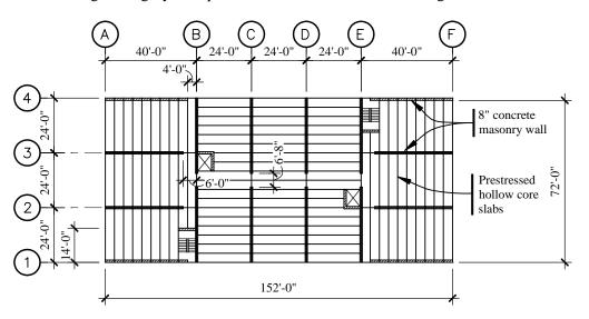
**Figure 9.2-1** Typical floor plan (1.0 in = 25.4 mm, 1.0 ft = 0.3048 m).
