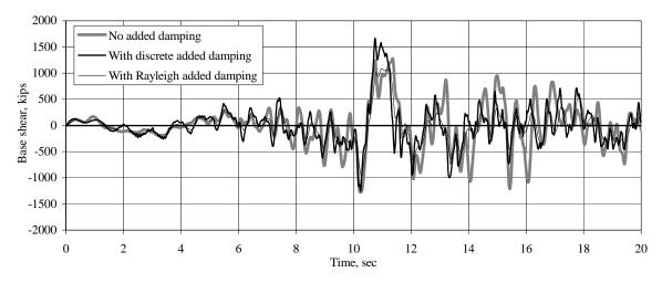
Figure 1Figure 3.2-71 Base shear time histories obtained from column forces (1.0 kip = 4.45 kN).
