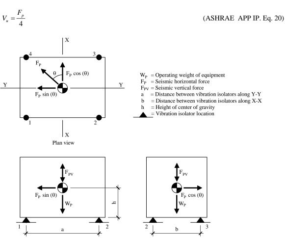
Figure 13.3-4 ASHRAE diagonal seismic force analysis for vibration isolation springs.
