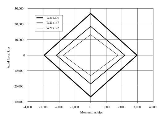
Figure 3.2-21 Yield surface used for modeling columns.
