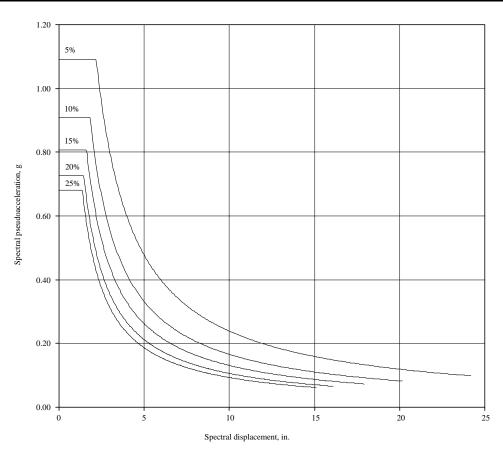
Figure 3.2-40 Demand spectra for several equivalent viscous damping values.
