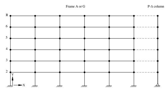
Figure 3.2-4 Simple wire frame model used for preliminary analysis.
