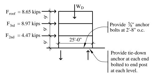
**Figure 10.1-9** Transverse wall: overturning (1.0 ft = 0.3048 m, 1.0 in. = 25.4 mm, 1.0 kip = 4.45 kN).
