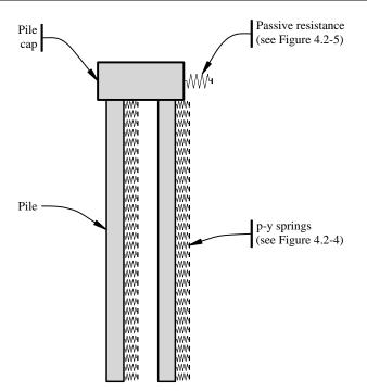
Figure 4.2-2 Schematic model of deep foundation system.
