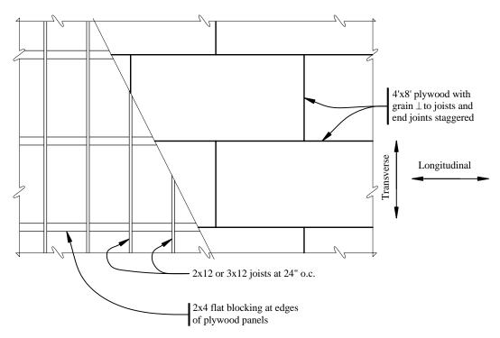
**Figure 10.2-3** Plywood layout (1.0 ft = 0.3048 m, 1.0 in. = 25.4 mm).
