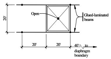
Figure 10.2-6 Diaphragm at roof opening (1.0 ft = 0.3048 m).
