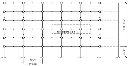
Figure 3.2-7 Detailed analytical model of 6-story frame.
