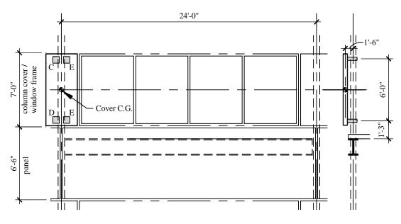
**Figure 13.2-6** Column cover connection layout (1.0 ft = 0.3048 m).
