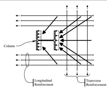
Figure 8-16 Force transfer from deck to column.
