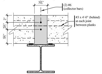
**Figure 7.1-4** Interior joint reinforcement at the ends of plank and the collector reinforcement at the end of the interior longitudinal walls - Joints 1 and 5 (1.0 in. = 25.4 mm).
