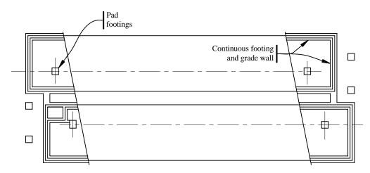
Figure 10.1-3 Foundation plan.
