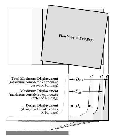
Figure 11.3-2 Design, maximum, and total maximum displacement.
