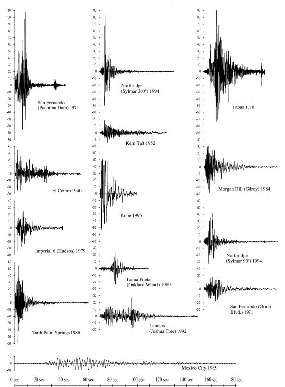
**Figure 1.2-1** Earthquake ground acceleration in epicentral regions (all accelerograms are plotted to the same scale for time and acceleration). Great earthquakes extend for much longer periods of time.
