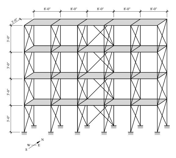
Figure 12-3 Steel storage rack (1.0 ft = 0.3048 m).
