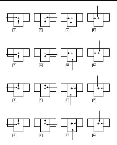
Figure 3.1-8 Basic load cases used in ELF analysis.
