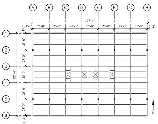
Figure 4.1-1 Typical framing plan.
