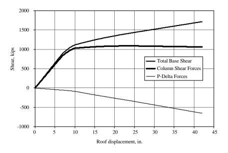
Figure 3.2-22 Two base shear components of pushover response.
