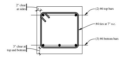
Figure 4.2-18 Foundation tie section.
