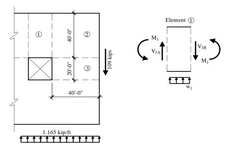
Figure 10.2-7 Chord forces and Element 1 free-body diagram (1.0 ft = 0.3048 m, 1.0 kip = 4.45 kN, 1.0 kip/ft = 14.6 kN/m).
