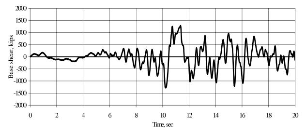
Figure 3.2-57 Time history of total base shear, Ground Motion A00, including P-delta effects.
