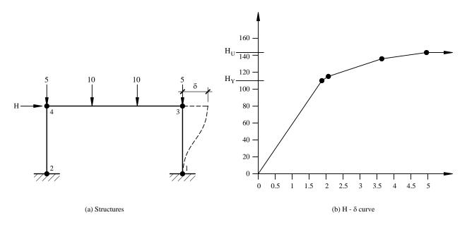
**Figure 1.2-6** Initial yield load and failure load for a ductile portal frame. The margin from initial yield to failure (mechanism in this case) is known as overstrength.
