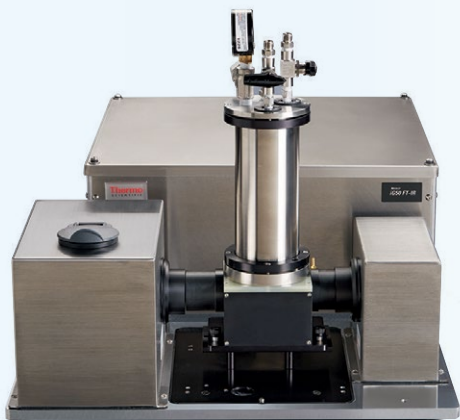
Extended sample compartment with 10 meter gas cell
