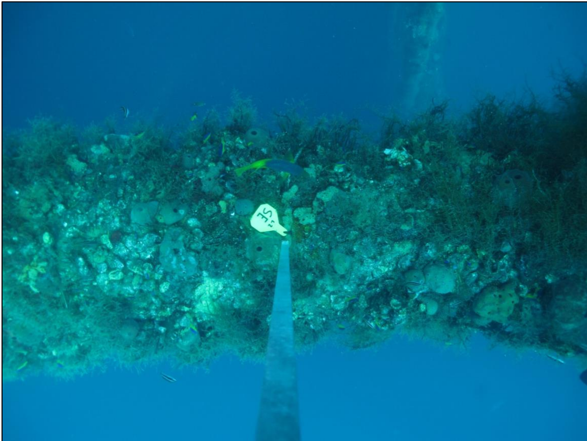
Figure 2.10. Repetitive photostation with camera mounted above aluminum t-frame. Photo: NOAA
