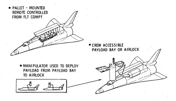
Figure 1-4. Shuttle Payload Accommodations
