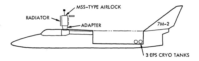
Figure 6-7. 7M-2 Payload General Arrangement
