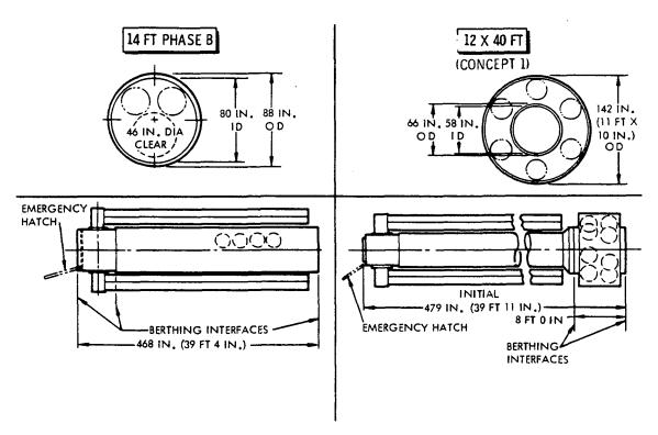
Figure 7. Special Module (Power)
