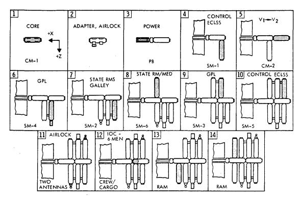
Figure 36. 12-Foot Module Initial MSS Buildup Sequence
