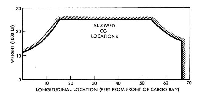
Figure 2-8. Payload Center-of-gravity Envelope
