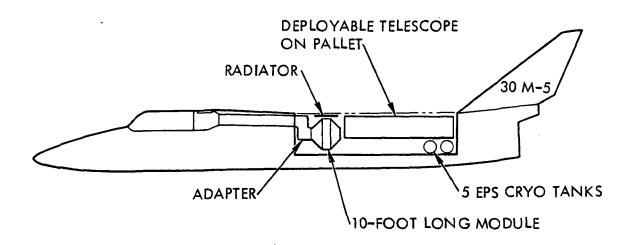
Figure 6-16. 30M-5 Payload General Arrangement
