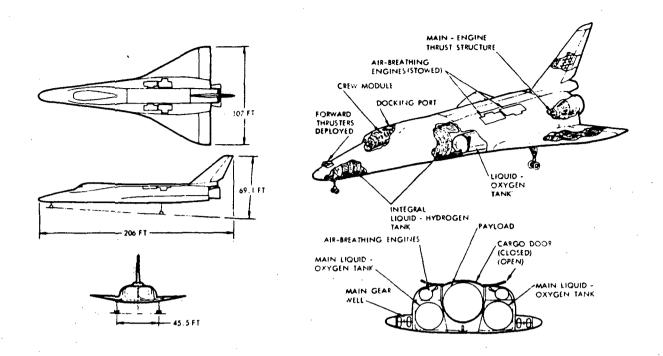
Figure 2-7. Orbiter Configuration
