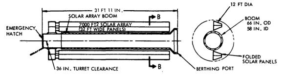
• GROWTH STATION 10,000 FT<sup>2</sup> SOLAR ARRAY - 38. 3 FT OVERALL LENGTH DELTA EQUIPMENT
