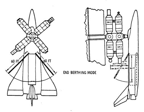
Figure 38. Shuttle/Station Berthing Mode - Initial Station, 14-Foot Diameter
