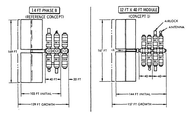
Figure 2. Reduced Payload Size Concept Dimensions
