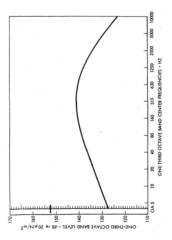
Figure B-1. Cargo Bay Acoustic Spectrum
