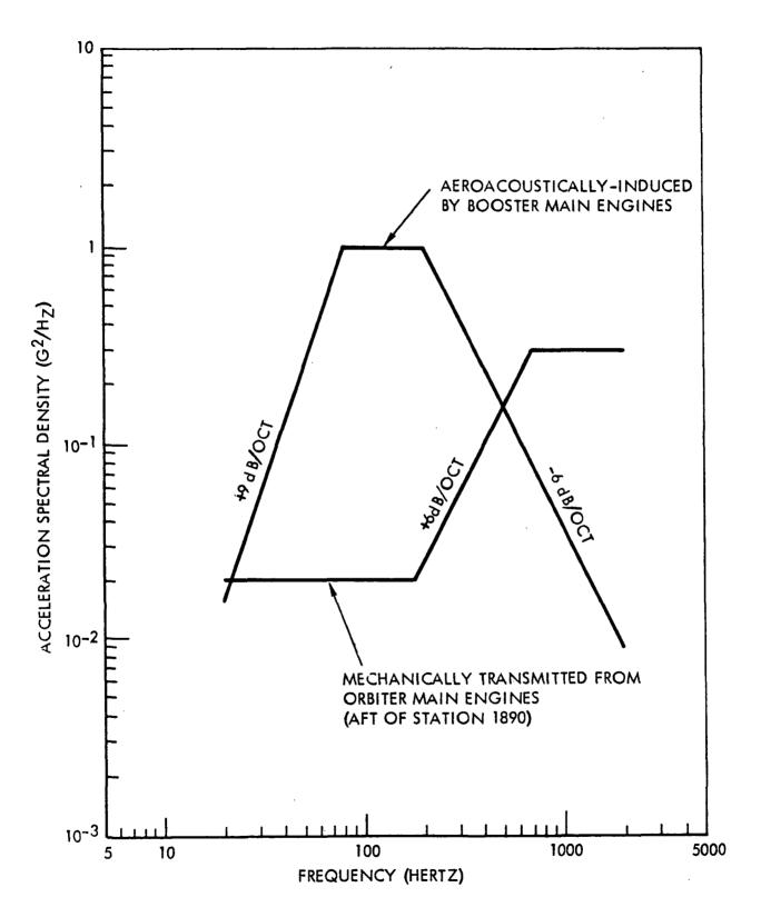
Figure B-2. Cargo Bay Vibration Spectra
