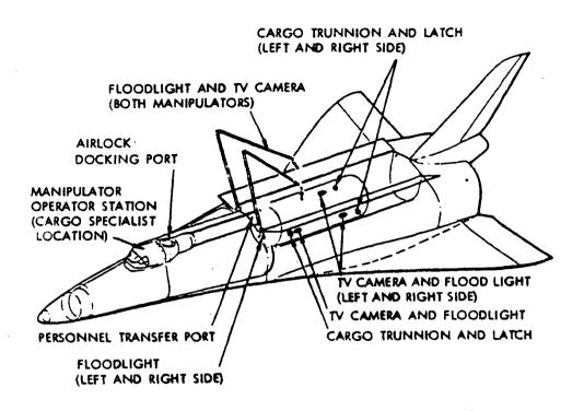
Figure 2-10. Docking and Payload Handling System
