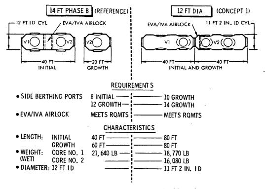
Figure 9. Special Module (Core)
