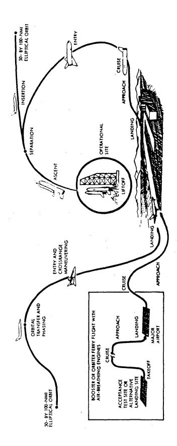
Figure 2-1. Shuttle Operational Sequence
