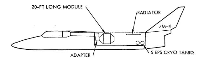
Figure 6-9. 7M-4 Payload General Arrangement
