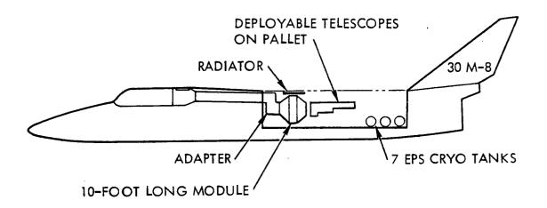
Figure 6-19. 30M-8 Payload General Arrangement
