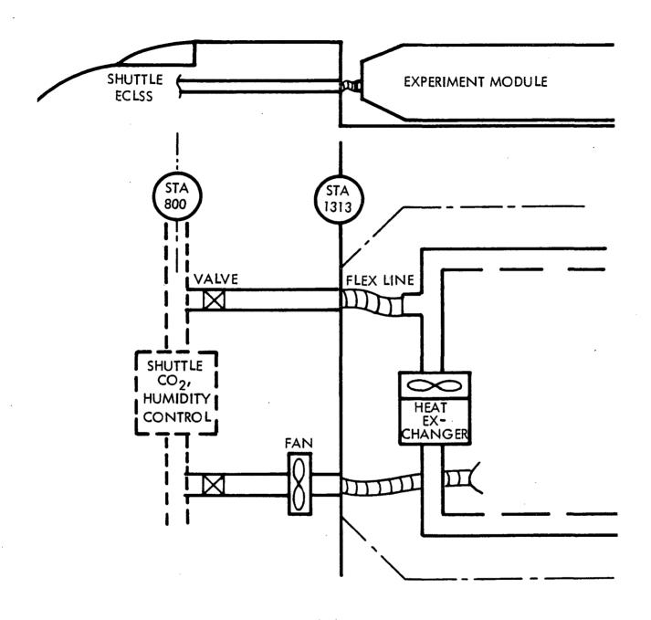
Figure 5-4. Sortie ECLSS Ducting
