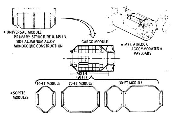
Figure 1-8. Structure Concept Selection
