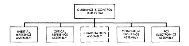
Figure 33. Guidance and Control Subsystem (G&C)
