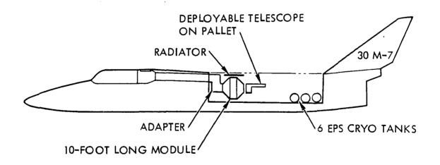
Figure 6-18. 30M-7 Payload General Arrangement
