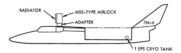
Figure 6-11. 7M-6 Payload General Arrangement
