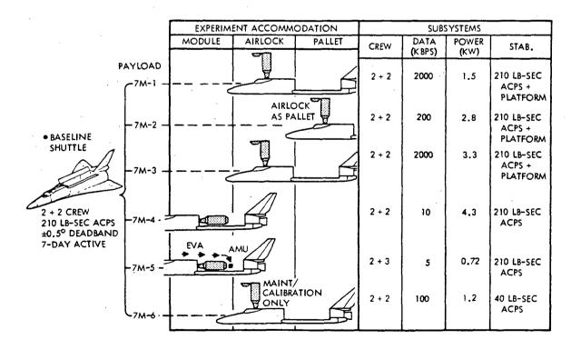
Figure 1-6. 7-Day Mission Payload Characteristics
