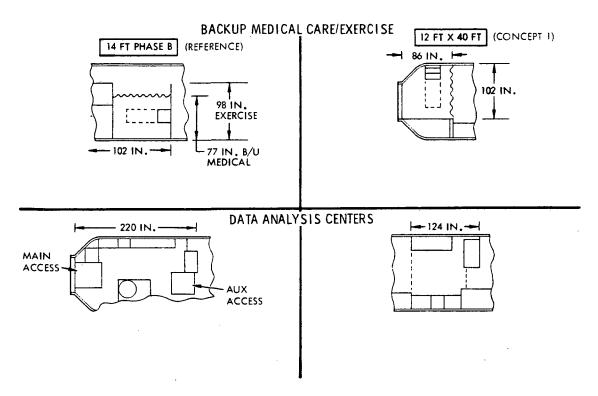
Figure 15. Station Module Facilities - Backup Medical Data Analysis
