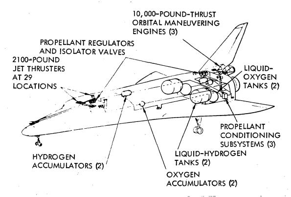
Figure 2-11. Auxiliary Propulsion System
