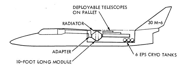
Figure 6-17. 30M-6 Payload General Arrangement
