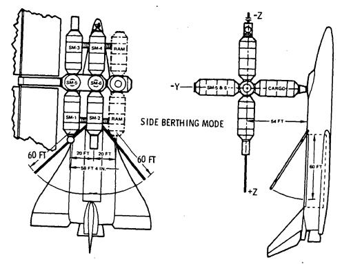
Figure 39. Shuttle/Station Berthing Mode - Growth Station, 14-Foot Diameter
