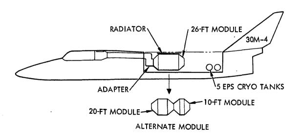
Figure 6-15. 30M-4 Payload General Arrangement
