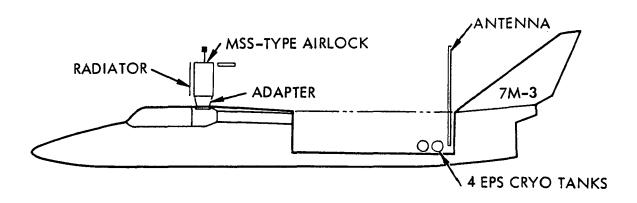
Figure 6-8. 7M-3 Payload General Arrangement
