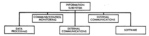
Figure 34. Information Subsystem (ISS)
