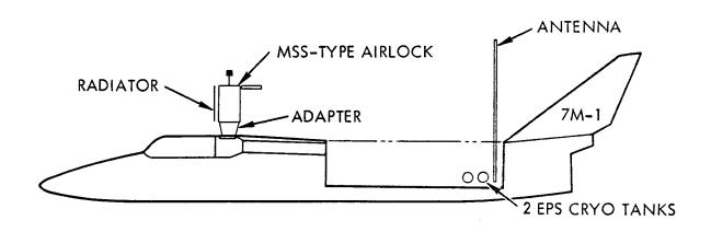
Figure 6-6. 7M-1 Payload General Arrangement
