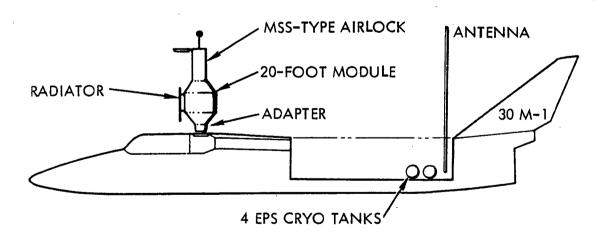
Figure 6-12. 30M-1 Payload General Arrangement
