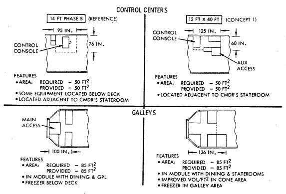
Figure 13. Station Module Facilities
