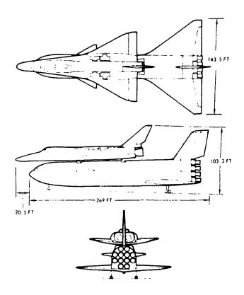
Figure 2-6. Mated Vehicle Configuration
