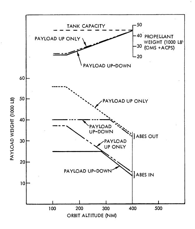
Figure 4-4. Payload Capability-Propellant Requirements: 55° Inclination Angle
