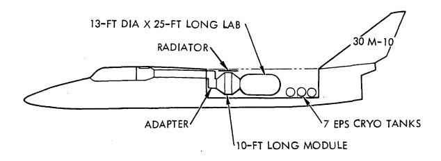
Figure 6-21. 30M-10 Payload General Arrangement
