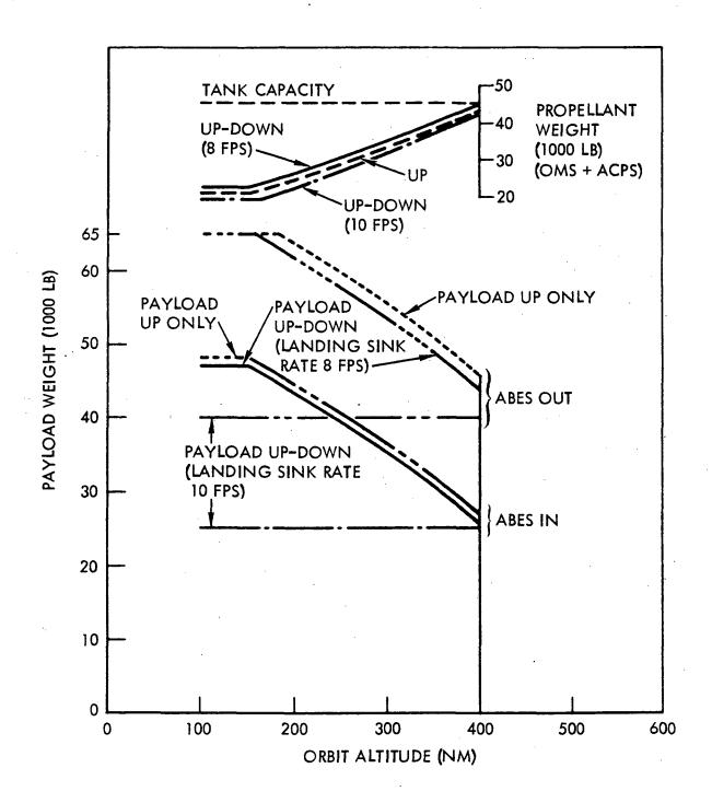
Figure 4-3. Payload Capability-Propellant Requirements: 28.5° Inclination Angle
