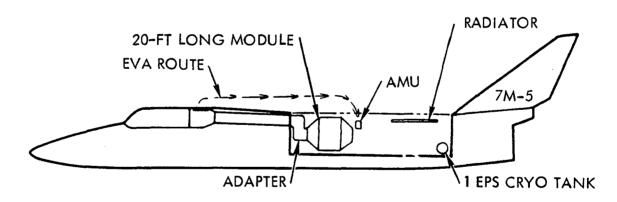
Figure 6-10. 7M-5 Payload General Arrangement
