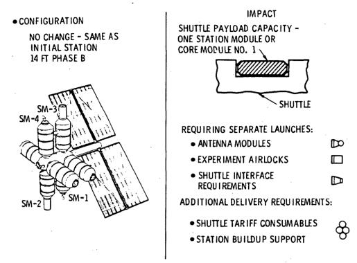
Figure 20. Reduced Payload Bay Length Impact - Concept 2 (14- by 40-Foot Modules)
