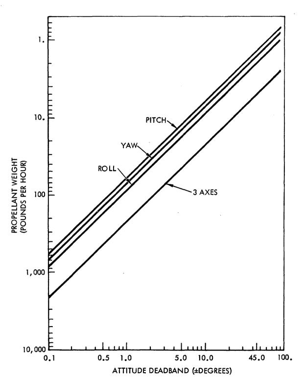
Figure 4-6. Attitude Hold, ACPS Propellant Requirement
