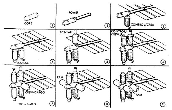
Figure 35. MSS Buildup Sequence-14-Foot Phase B
