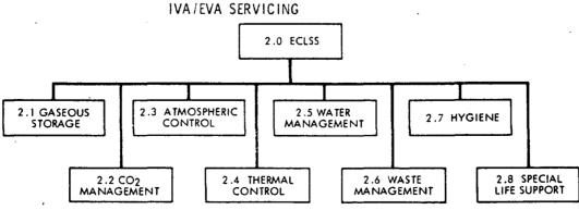
Figure 29. Environmental Control and Life Support Subsystem (ECLSS)
