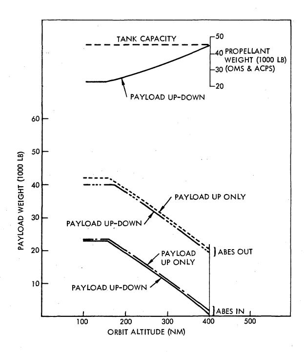
Figure 4-5. Payload Capability-Propellant Requirements: 90° Inclination Angle
