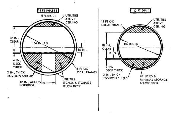
Figure 10. Station Modules - Cross Section Arrangement
