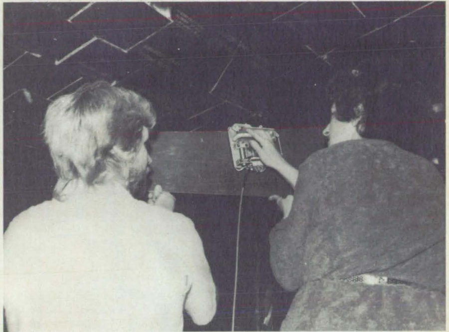
Figure 1. An Operator Moves the Carriage of the contour-measuring device on a beamlike track. A stylus on the carriage traces the contour of the surface above it.
