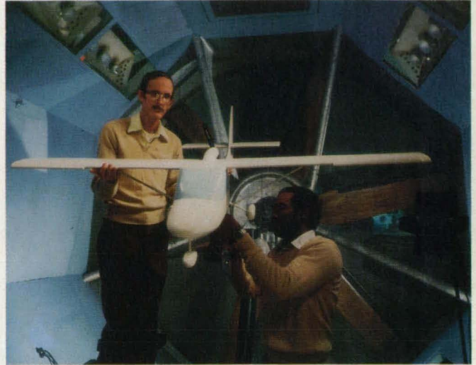
A NASA-developed wing design featuring drooping extensions on the outboard leading edges could help reduce the number of aviation accidents caused by stalling and spinning. After extensive studies at NASA's Langley Research Center, the design is now being put to the test on a new lightweight airplane. See Mission Accomplished, page 109.
