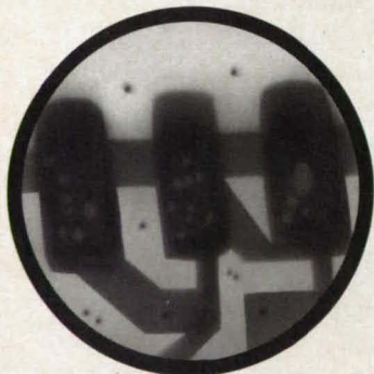
Detecting solder voids and solder balls under leadless carrier in a surface mount device.
