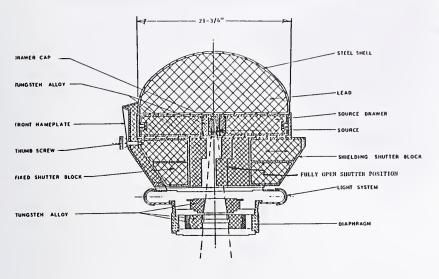
7.7.3.1 Vertical Beam <sup>60</sup>Co Source - This source consists of a single capsule containing about 7
