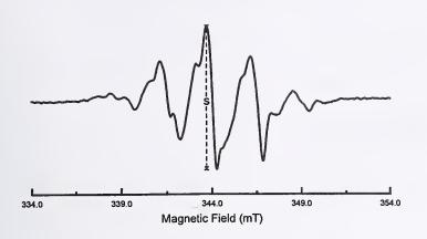
Figure 6 - Electron Paramagnetic Resonance Spectrum of Alanine
