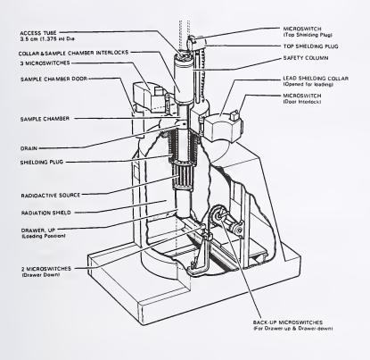
Figure 4 - Gammacell 220 60Co Irradiator
