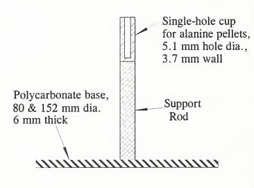
Figure 9 - Single-Hole Geometry for Alanine Pellets in High-Dose Rate Irradiators
