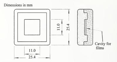
Figure 11 - Holder for Radiochromic Thin Film Irradiation
