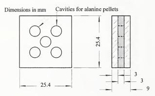
Figure 12 - Holder for Alanine Pellets to Simulate Thin Film Holder Geometry
