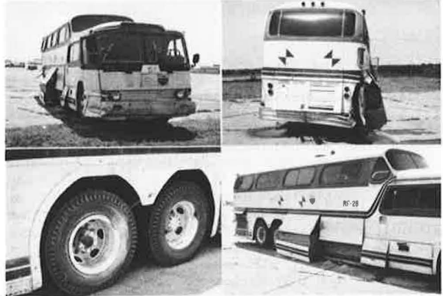
Figure 9. Vehicle damage, test RF-28.
