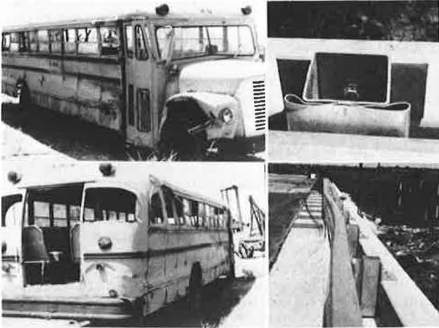
Figure 6. Vehicle and barrier damage, test RF-26.
