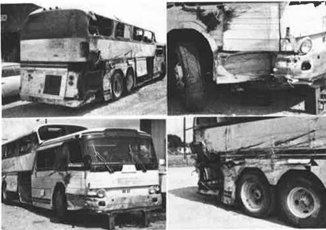
Figure 7. Vehicle damage, test RF-27.
