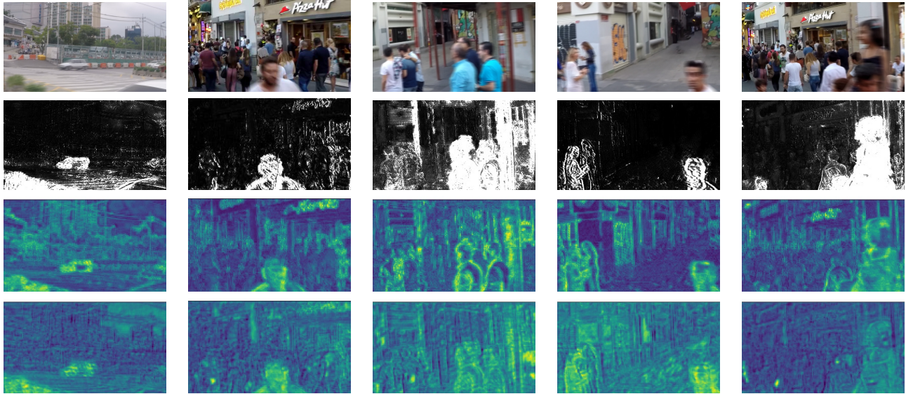
Figure 7. The second row shows one of the spatial attention map for each image. The third row shows the spatial distribution of the horizontal-offset values for the filter. Fourth row shows the variance of the predicted kernel values.
