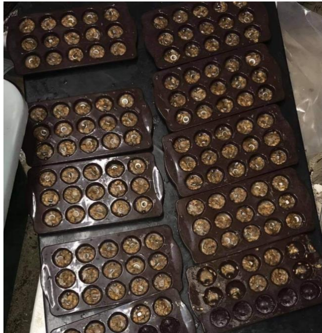
Figure 28: Example of food preparation. 2 g feeding blocks consisting of mussels 87.5% mussel and 2.5% MP frozen in chocolate moulds. The food blocks were negatively weighted with a stainless steel nut
